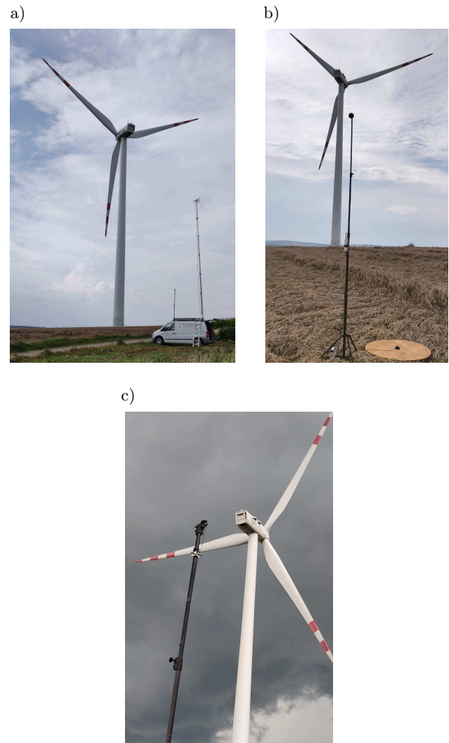
Fig. 4. Location of acoustic measurement positions near the Gamesa G87 turbine in Orzechowce: a) point 1, b) point 2, c) point 3.
