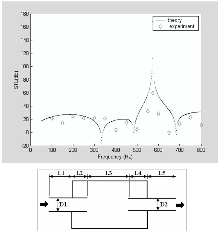
Fig. 6. Performance of a single-chamber muffler with extended tubes at the zero mean flow velocity [ $D_1 = D_2 = 0.054$  (m),  $L_1 = L_5 = 0.175$  (m),  $L_2 = L_4 = 0.150$  (m),  $L_3 = 0.504$  (m)] [experimental data is from CHIU *et al.* (2006)].
