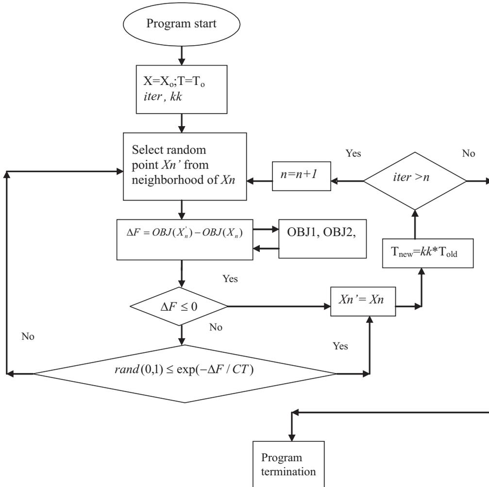
Fig. 8. Flow diagram of a *SA* optimization.
