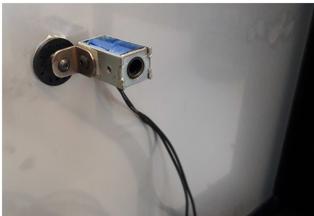
Fig. 4. Solenoid with inductor mounted at the centre of the incident panel.
