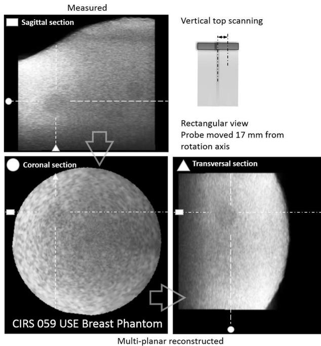
Fig. 14. Images of selected CIRS 059 USE breast phantom sections acquired using vertical top scanning with the rectangular view and the probe moved 17 mm from rotation axis.
