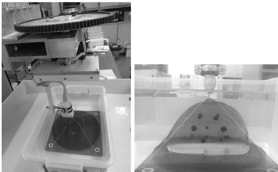
Fig. 8. Measurement system used in multi-angle conventional ultrasound imaging (MACUI).
