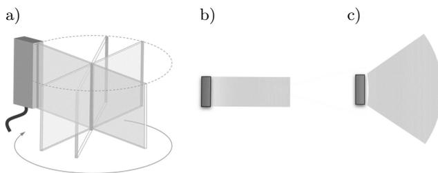
Fig. 9. The vertical lateral configuration applied in the MACUI method with different views: a) vertical lateral scanning, b) rectangular view, c) sectoral view.
