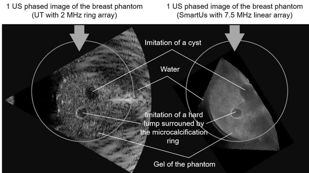
Fig. 4. Images of the same coronal section fragment of the Model B-MM – 1.2 Yezitronix breast phantom obtained by means of the 32-element subarray of the ultrasound tomography ring array (2 MHz) with linear phased mode scanning, and by means of the conventional linear array (7.5 MHz) of the SmartUs Telemed B-mode scanner with virtual convex scanning (courtesy of DRAMIŃSKI S.A. company).
