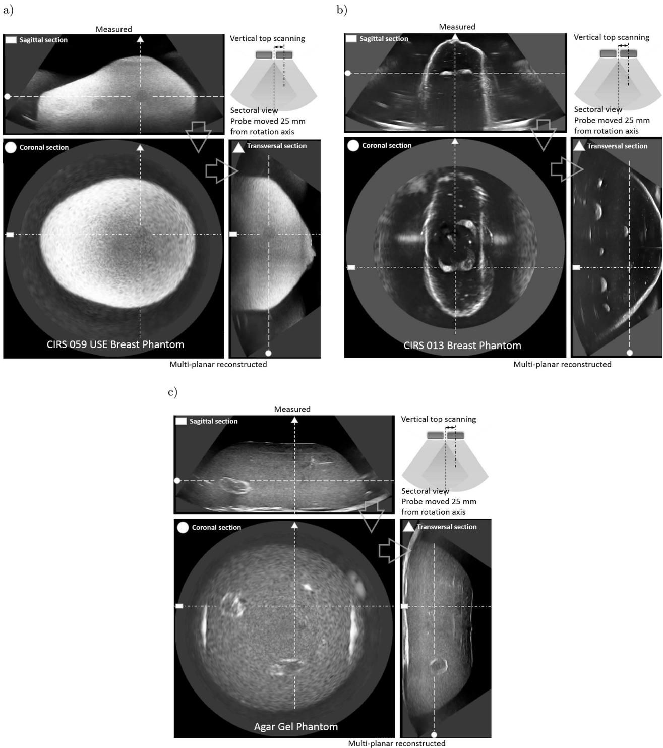
Fig. 15. Images of selected breast phantom sections acquired using vertical top scanning with the sectoral view and the probe moved 25 mm from rotation axis: a) CIRS Model 059 USE Phantom, b) CIRS 013 Mammography Phantom, c) self-made Agar Gel Phantom.
