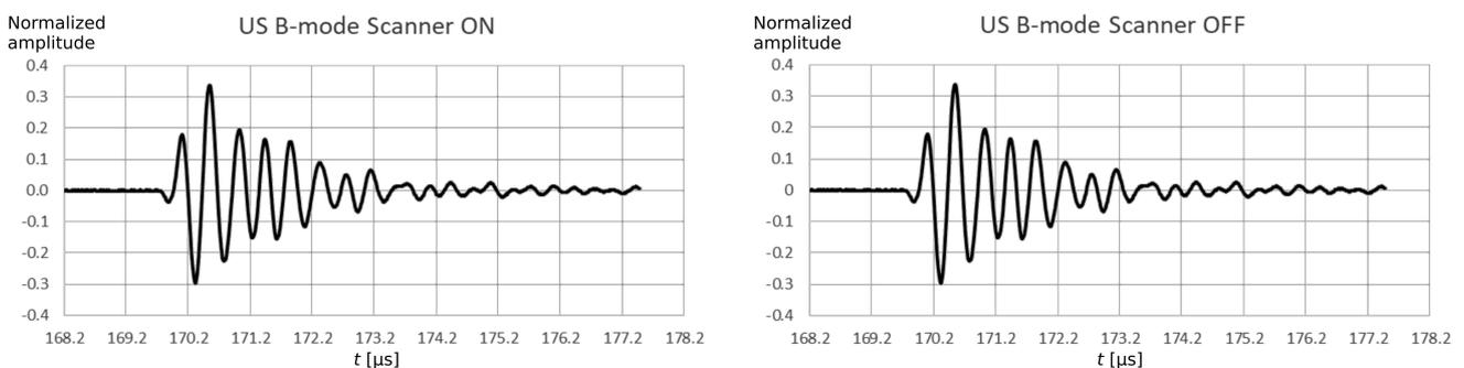
Fig. 17. The pulses transmitted through the medium as presented in Fig. 16 when the ultrasound B-mode scanner is ON and OFF.
