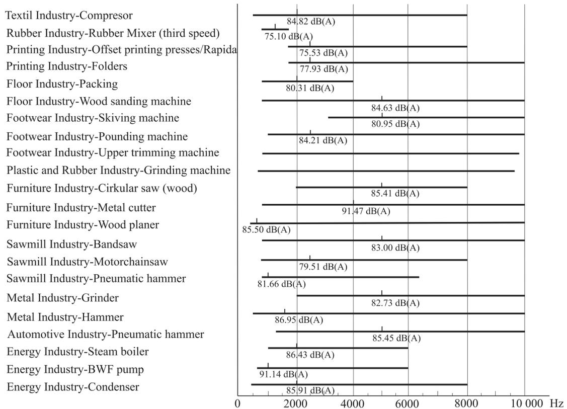
Fig. 4. Means of  $L_{eq}$  levels for machines that exceeded N-80 curve levels.
