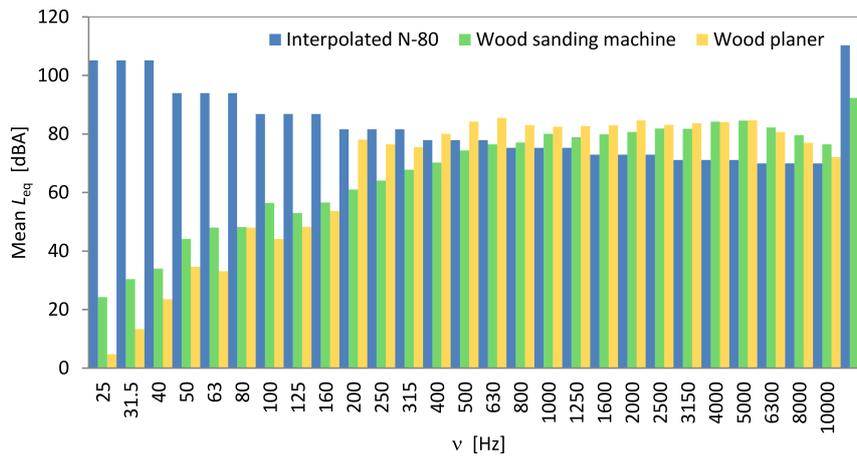
Fig. 6. Means of  $L_{eq}$  at 1/3 octave bands for wood processing in comparison with the interpolated N-80 curve.
