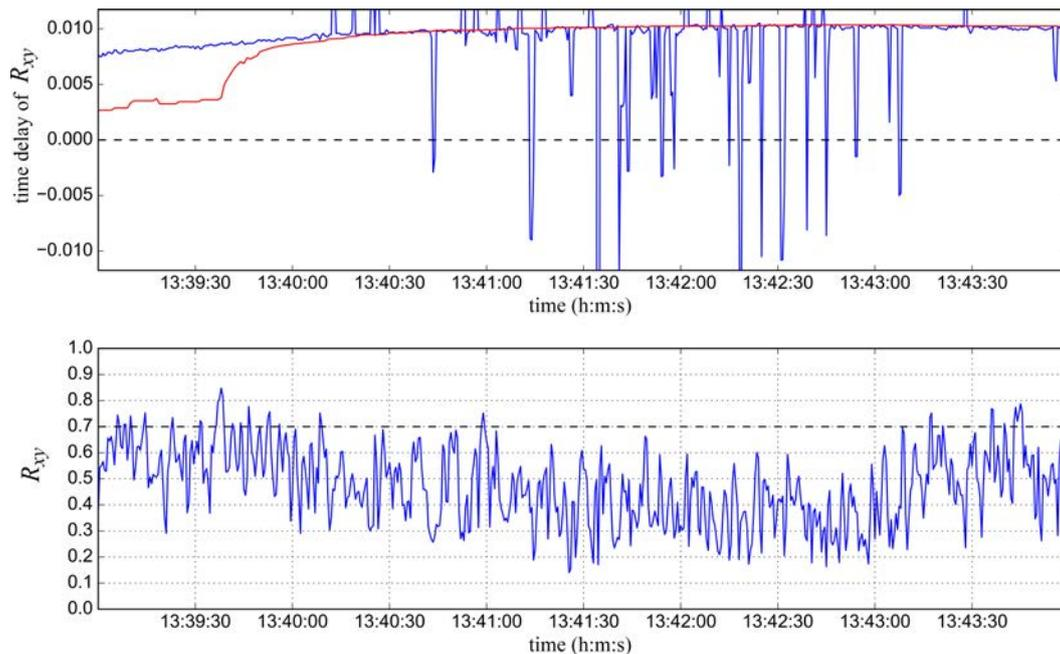
Fig. 7. Time delays of maxima of cross-correlation function (blue) with time delays calculated by GPS data (red) – upper diagram; and the value of coefficient of normalized cross-correlation function  $R_{xy}$  as a dependence on local time of the day – bottom diagram.
