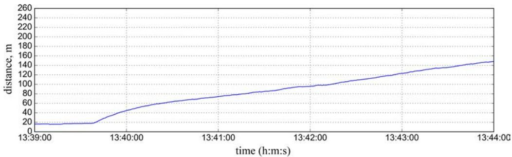
Fig. 6. GPS distance between the diver (towed buoy) and the center point of the pair of hydrophones 2, 7 as a dependence on local time of the day.
