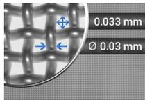
Fig. 6. Steel mesh used for the regenerator: surface area 0.033 mm<sup>2</sup>, diameter 0.03 mm.
