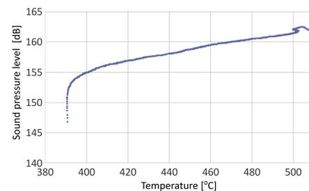
Fig. 12. The dependence of the sound pressure level on the temperature on the hot heat exchanger for a constant pressure in the waveguide of 6.6 bar – working medium argon.
