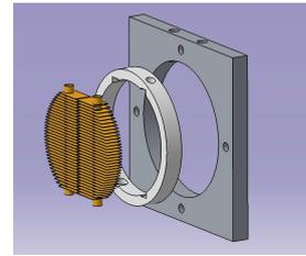
Fig. 7. Thermal isolation – hot heat exchanger.
