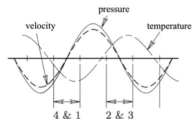
Fig. 2. Waveforms of pressure, acoustic velocity, and temperature as function of time for a travelling wave and  $r_h \simeq \delta_k$ .
