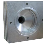
Fig. 4. Cross-section increase in the regenerator module.
