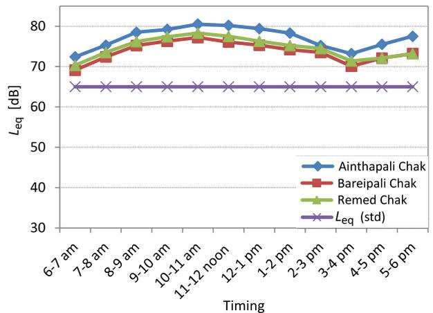
Fig. 8.  $L_{eq}$  at different locations (of commercial area on NH) during day hours.
