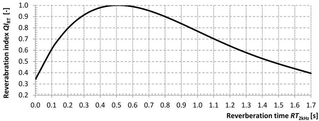
Fig. 4. Relationship between the reverberation time  $RT_{2\text{kHz}}$  and the reverberation index  $QI_{RT}$ .
