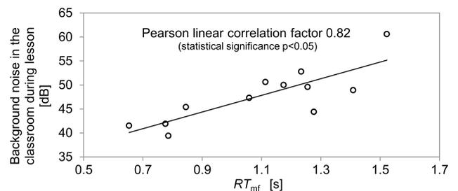
Fig. 1. Relationship between reverberation time  $RT_{mf}$  and the level of background noise during lessons (MIKULSKI, RADOSZ, 2012), where  $RT_{mf}$  is the arithmetic mean of the reverberation time from 500 Hz, 1000 Hz and 2000 Hz octave bands.
