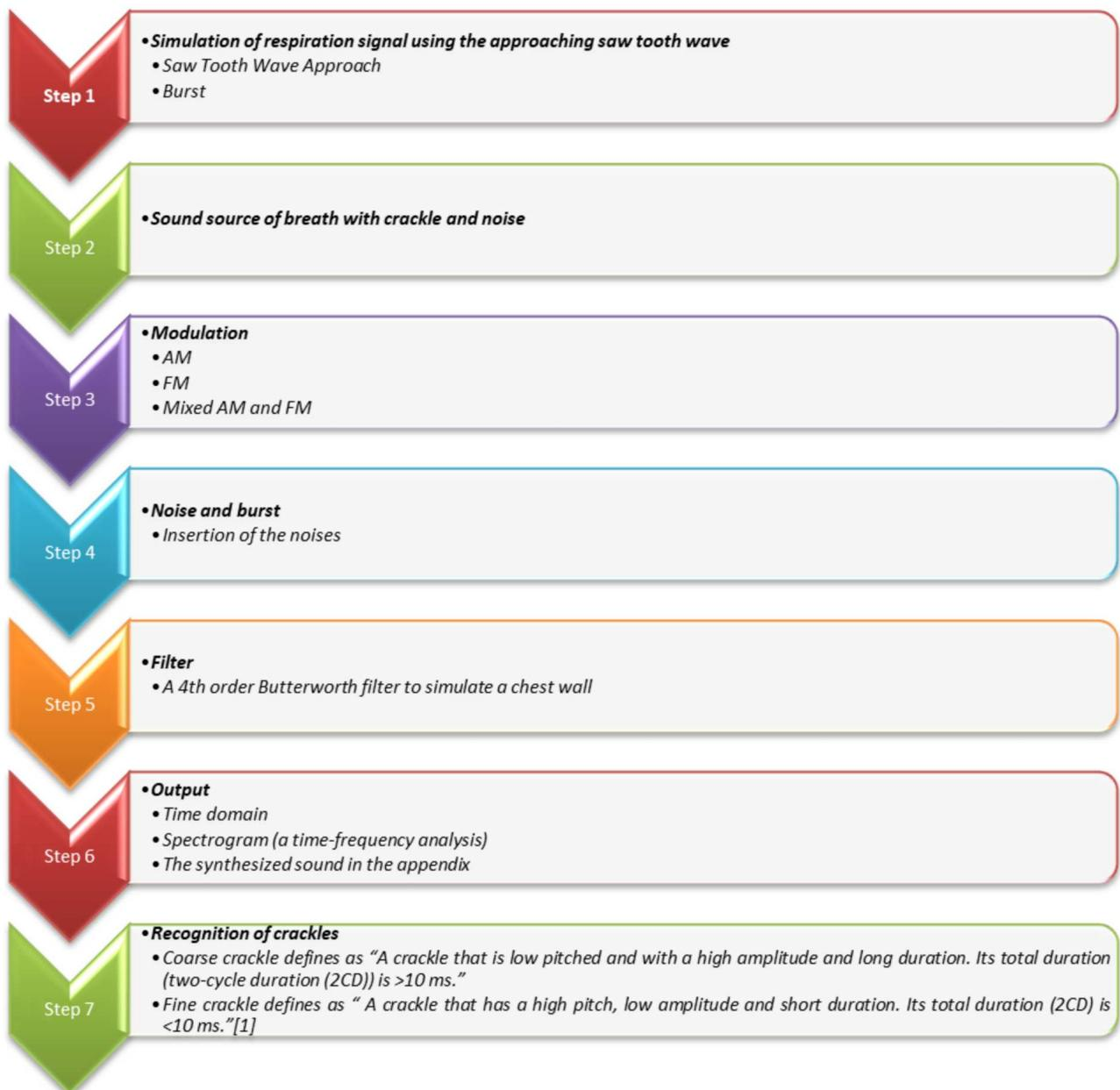
Fig. 1. Flow chart of the simulation processes for the communication model of crackles.
