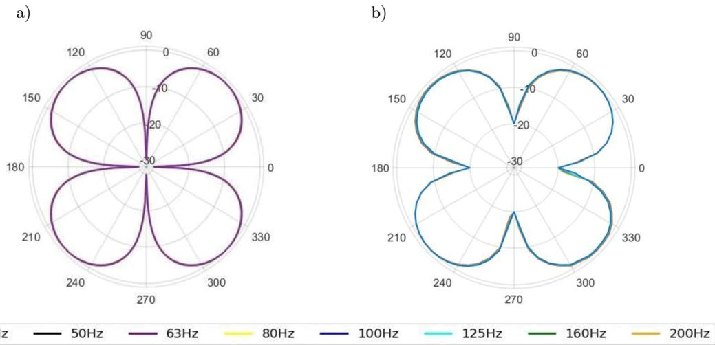
Fig. 5. Lateral quadrupole theoretical radiation: a) analytical, for the far field at 14 m, b) numerical, for the near field at 2 m. There is no distinction between the different frequencies.
