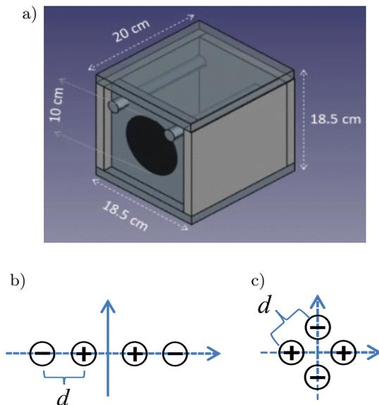
Fig. 1. Model of the designed bass-reflex system for a 4" low- $Bl$  driver (a). Schematic diagrams of longitudinal (b) and lateral (c) quadrupole compound sources.
