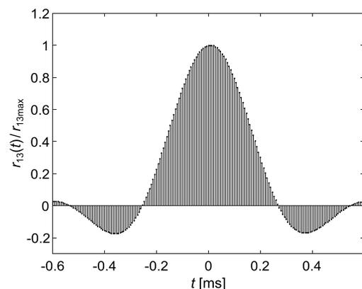
Fig. 8. Correlation function with hydrophone distance  $2d = 0.1$  m.
