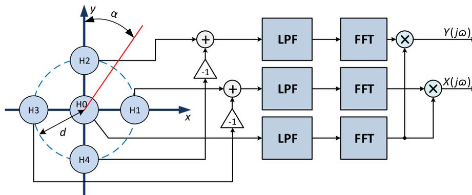
Fig. 1. Functional diagram of a DIFAR system.
