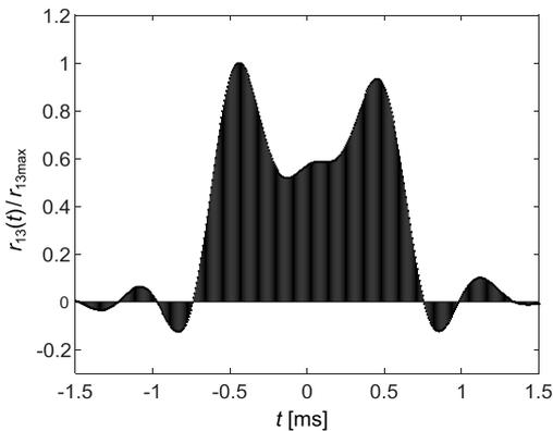
Fig. 11. Correlation function with hydrophone distance  $2d = 0.8$  m.
