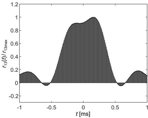
Fig. 9. Correlation function with hydrophone distance  $2d = 0.4$  m.
