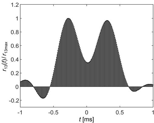
Fig. 10. Correlation function with hydrophone distance  $2d = 0.6$  m.
