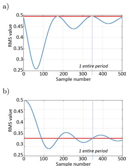
Fig. 5. Dependence of the RMS value of the signal on the DFT length expressed in the number of samples: a) the initial phase equal to 0.8 rad; b) initial phase equal to 0. Theoretical effective value of the sinusoidal signal is marked with a red line.
