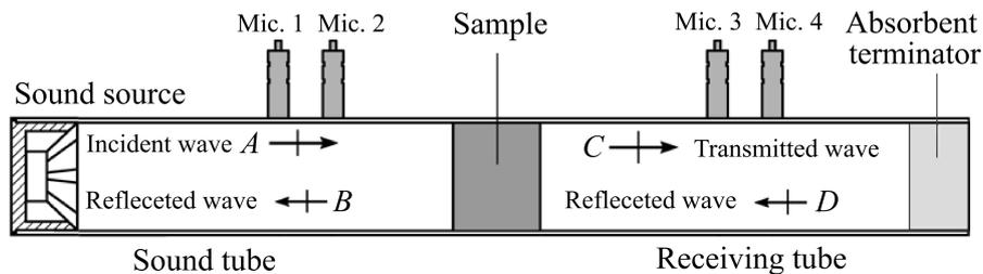
Fig. 3. Transmission Loss experimental setup.
