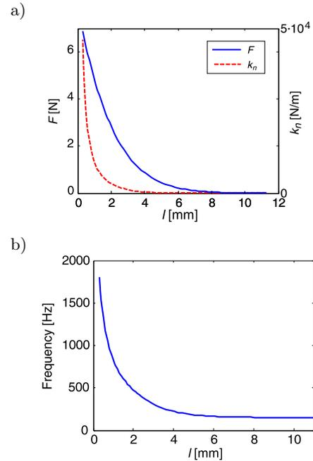
Fig. 2. a) Measured static magnetic force  $F$  exerted on the rigid iron platelet, and  $k_n$  obtained according to  $F$ ; b) predicted first anti-resonance frequencies plotted against relative distance  $l$ .
