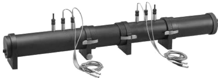
Fig. 4. The Bruel and Kjaer Transmission Loss Type 4206.
