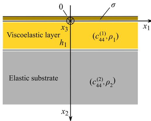
Fig. 1. Cross-section of the analysed Love wave waveguide loaded with a surface mass density  $\sigma$ . Love surface waves propagate along the  $x_1$  axis. Shear horizontal (SH) mechanical displacement  $u_3$  of the Love wave is directed along the  $x_3$  axis.
