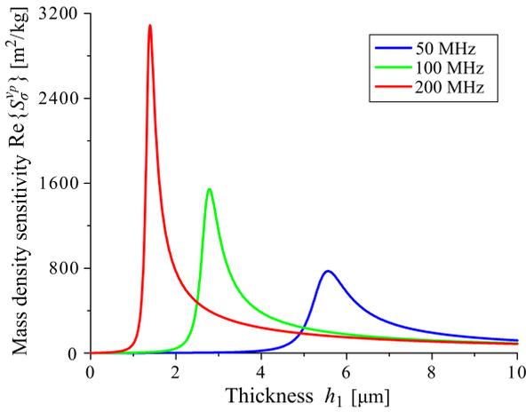
Fig. 3. Real part of the mass density sensitivity  $S_{\sigma}^{vp}$  [ $\text{m}^2/\text{kg}$ ] for Love surface waves propagating in PMMA-ST – Quartz waveguides, loaded with a thin lossless film with the mass density  $\sigma$ , as a function of thickness  $h_1$  of the PMMA guiding surface layer, for different values of wave frequency  $f = 50, 100,$  and  $200$  MHz.
