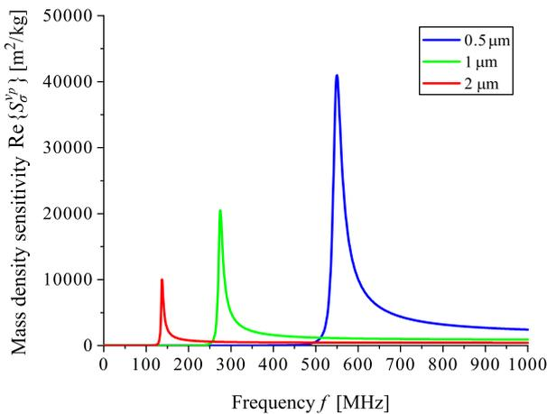
Fig. 4. Real part of the mass density sensitivity  $S_{\sigma}^{vp}$  [ $\text{m}^2/\text{kg}$ ] for Love surface waves propagating in PMMA – Diamond waveguides loaded with a thin lossless film with the mass surface density  $\sigma$ , as a function of Love wave frequency  $f$ , for different values of thickness  $h_1$  of the guiding PMMA surface layer ( $h_1 = 0.5, 1,$  and  $2$   $\mu\text{m}$ ).
