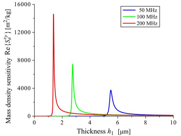
Fig. 5. Real part of the mass density sensitivity  $S_{\sigma}^{vp}$  [ $\text{m}^2/\text{kg}$ ] for Love surface waves propagating in PMMA – Diamond waveguides, loaded with a thin lossless film with the surface mass density  $\sigma$ , as a function of thickness  $h_1$  of the PMMA guiding surface layer, for different values of wave frequency  $f = 50, 100,$  and  $200$  MHz.
