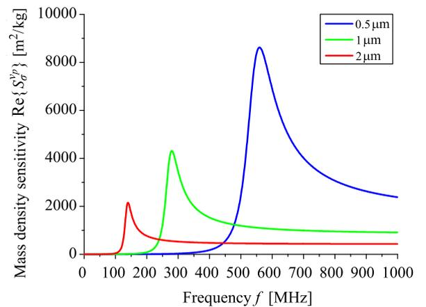
Fig. 2. Real part of the mass density sensitivity  $S_{\sigma}^{vp}$  [m<sup>2</sup>/kg] for Love surface waves propagating in PMMA-ST – Quartz waveguides loaded with a thin lossless film with the surface mass density  $\sigma$ , as a function of Love wave frequency  $f$ , for different values of thickness  $h_1$  of the guiding PMMA surface layer ( $h_1 = 0.5, 1, \text{ and } 2 \mu\text{m}$ ).
