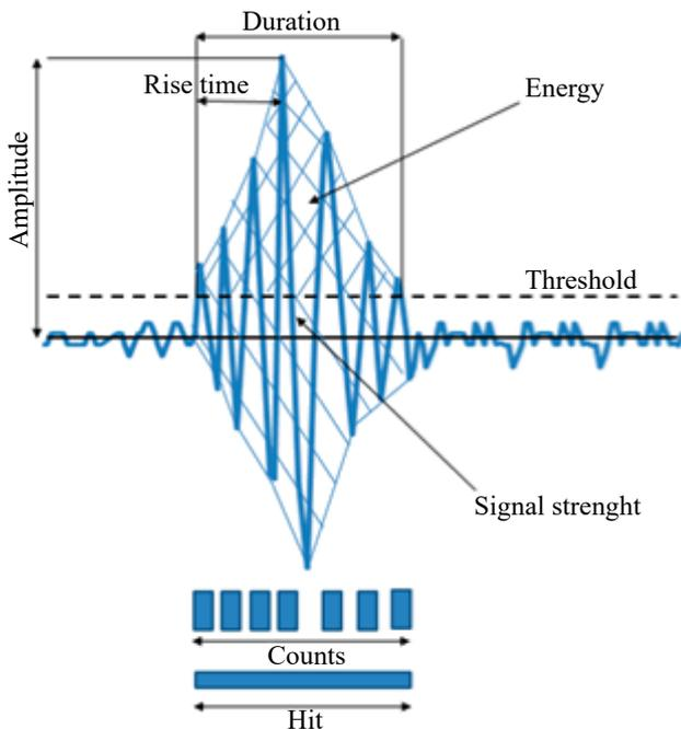
Fig. 5. Parameters reflecting of an AE waveform (ZAKI *et al.*, 2015).
