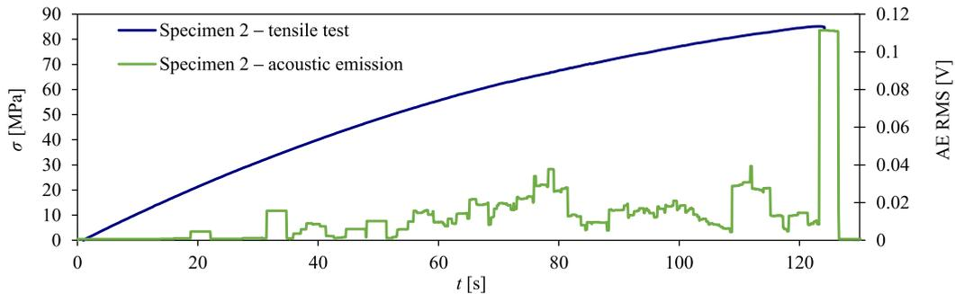
Fig. 12. Stress and RMS graph as a function of time for a sample with 10% polyester-glass recycle content.
