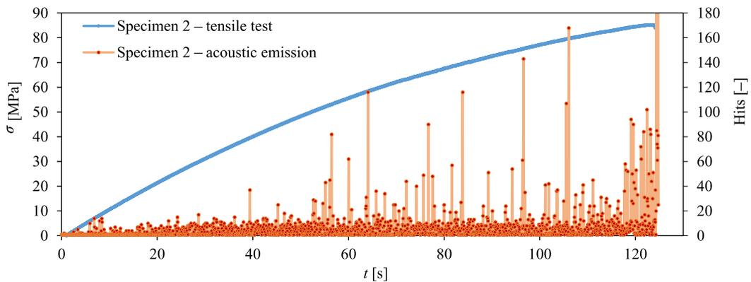
Fig. 7. Graph of stress and number of AE hits as a function of time for a selected sample with 10% recycle content.
