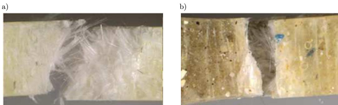
Fig. 10. Samples after static tensile testing:
