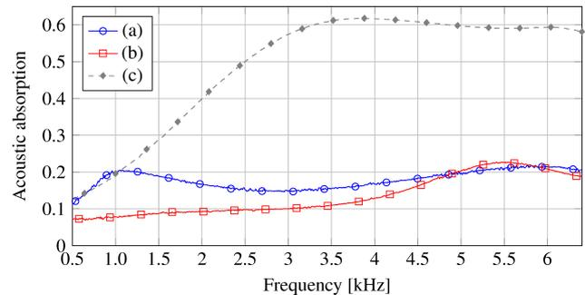
Fig. 8. Acoustic absorption of ceramic samples with porosity 72%: (a) thickness 16 mm, (b) thickness 22 mm. Acoustic absorption of stiff PU foam with porosity app. 98%: (c) thickness 26 mm.
