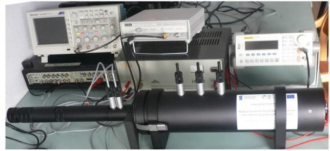
Fig. 4. Experimental setup for measurement of acoustic absorption coefficient of materials.
