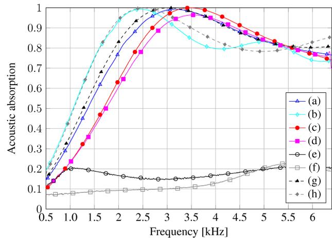
Fig. 9. Acoustic absorption of  $\text{Al}_2\text{O}_3$  ceramic samples with porosity: (a,b) 90%, (c,d) 88%, (e,f) 72%, (g,h) 89.5%; and thickness: (a) 18 mm, (b) 24 mm, (c) 14 mm, (d) 16.5 mm, (e) 16 mm, (f) 22 mm, (g) 18 mm, (h) 22 mm.
