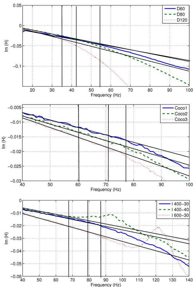
Fig. 5. Results of  $\text{Im}(H)$  as a function of frequency for three types of porous eco-materials; top: recycled foam, middle: coconut fibres, bottom: recycled polyester fibre. The vertical lines indicate the relevant upper frequency limits.
