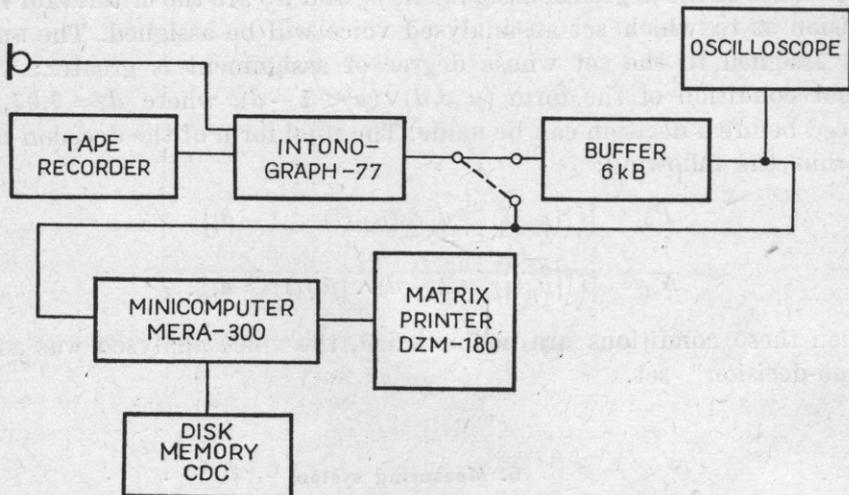
Fig. 3. A schematic block diagram of the measuring system used in the investigation
