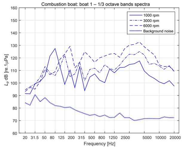
Fig. 18. 1/3 octave bands spectra combustion motor boat 1, for the three velocities evaluated. Background noise measured in the area is also shown.
