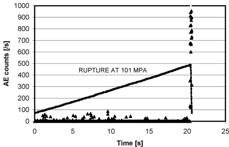
Fig. 2. Typical time dependence of AE counts (triangles) and applied bending stress (solid line) registered in investigated cordierite sample.
