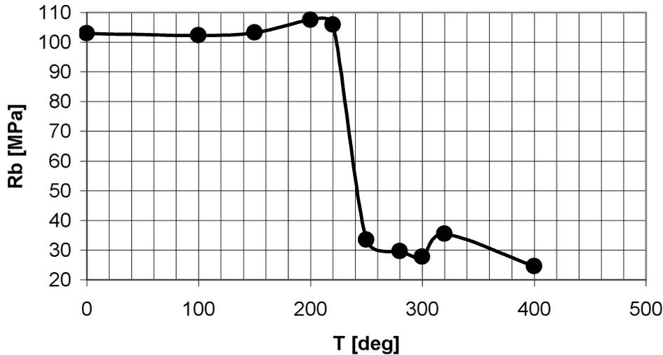
**Fig. 1.** Results of the measurements of three-point bending strength  $R_b$  for the cordierite samples, as a function of shocking temperature difference  $\Delta T$ , visible value of threshold shock temperature difference  $\Delta T_{\text{max}}$ .
