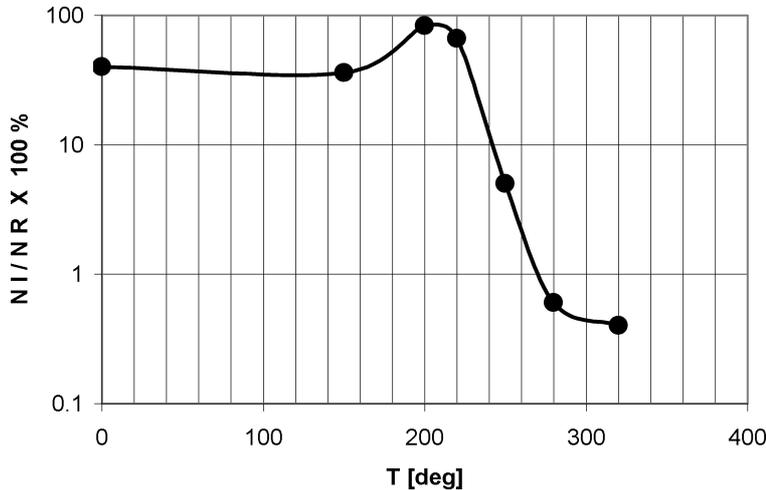
Fig. 3. The dependence  $N_I/N_R$  ratio on shocking temperature difference  $\Delta T$  for the investigated cordierite samples.
