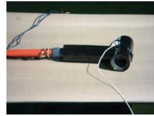
Fig. 3. View of the investigated T-type connector with a fastened AE sensor.
