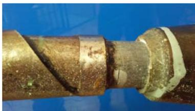
Fig. 2. Investigated cable termination with a partially removed insulating cover of the steel bandage.
