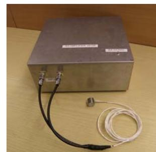
Fig. 4. View of the applied in-house made differential AE signal amplifier with the connected AE sensor of WD (Physical Acoustics Corporation) type.
