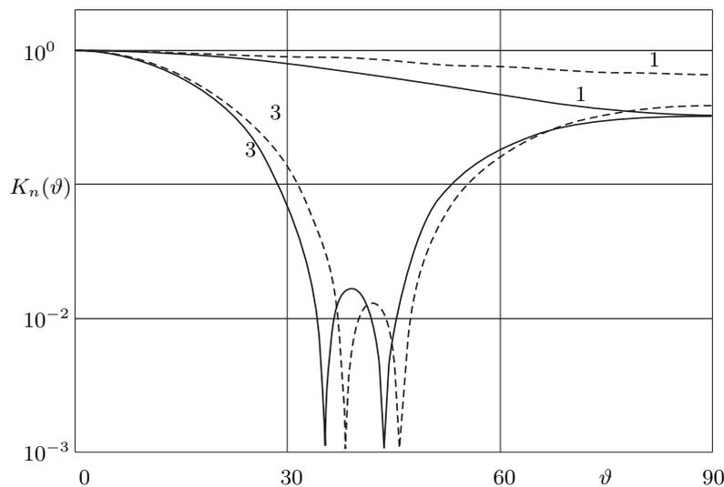
Fig. 3. Directional characteristics of annular source for  $s = 5$ ,  $\beta/x_n = 0.5$ ,  $n = 1$  and 3.
