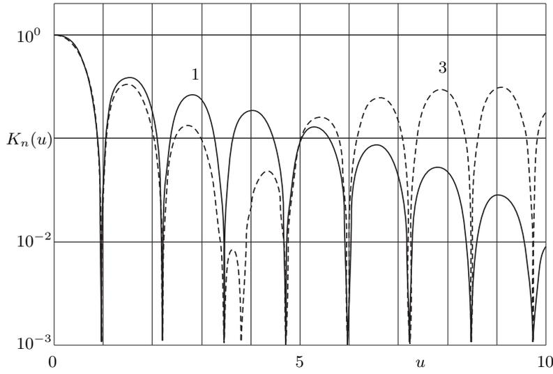
Fig. 5. Diagrams of  $K_n(u)$  function versus variable  $u = \beta \sin \vartheta$  for annular plate. It is assumed that  $s = 1.5$ ,  $n = 1$  and 3.
