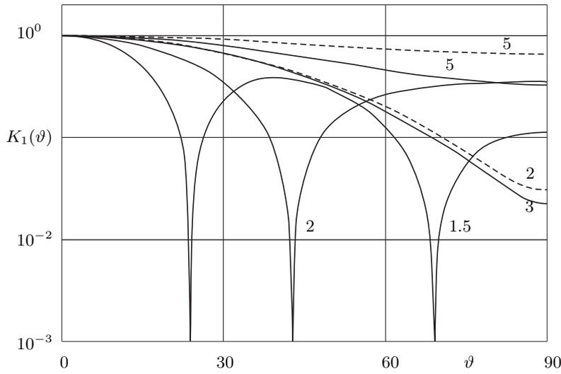
Fig. 1. Directional characteristics of annular source radiation for  $\beta/x_1 = 0.5$ ,  $s = 5, 3, 2$  and  $1.5$ . Attention for Figs. 1–4, 7: Curves in figures are: solid — vibrating plate is a source, dashed — vibrating membrane is a source.
