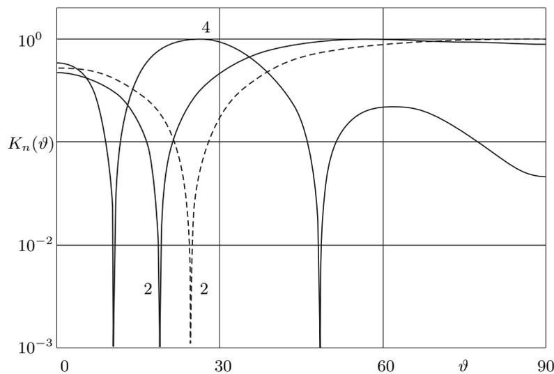
Fig. 4. Directional characteristics of annular source for  $s = 5$ ,  $\beta/x_n = 0.5$ ,  $n = 2$  and 4.
