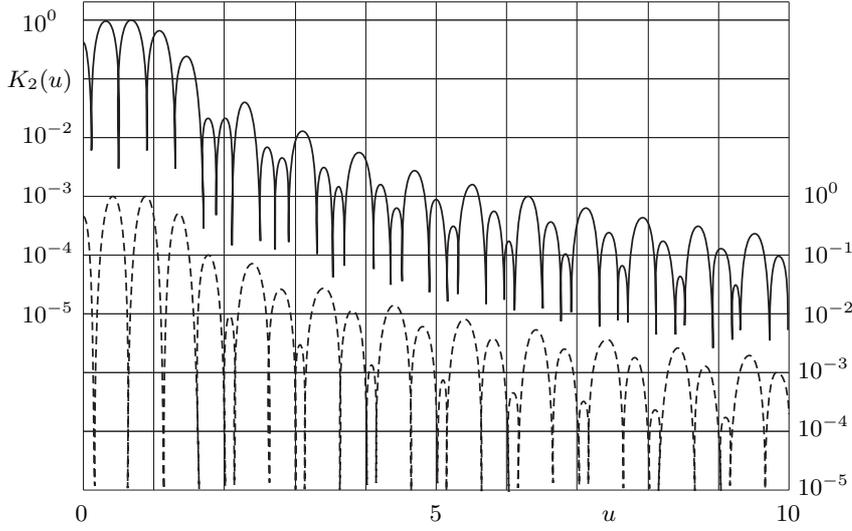
Fig. 7. Diagrams of  $K_2(u)$  function versus variable  $u = \beta/x_2 \sin \vartheta$  for annular source. It is assumed that  $s = 3$ .
