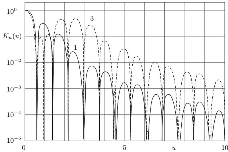
Fig. 6. Diagrams of  $K_n(u)$  function versus variable  $u = \beta \sin \vartheta$  for annular plate. It is assumed that  $s = 3$ ,  $n = 1$  and 3.
