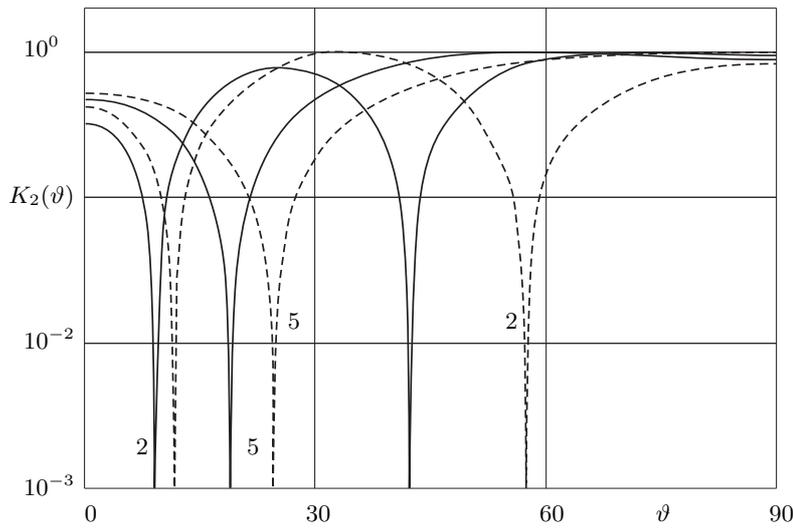
Fig. 2. Directional characteristics of annular source radiation for  $\beta/x_2 = 0.5$ ,  $s = 5$  and  $2$ .
