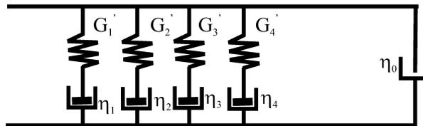
Fig. 2. The line of the independent Maxwell elements, as a model of a fluid with concentration of suspensions less than 0.1.
