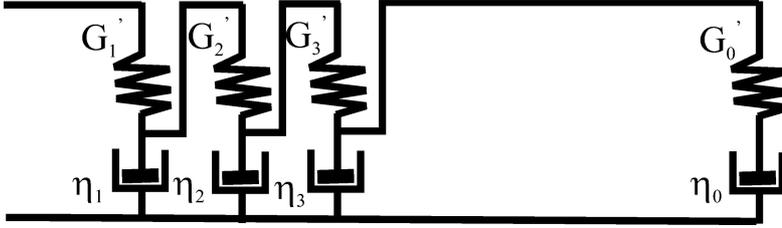
Fig. 3. The chain of coupled Maxwell elements, i.e. the “ladder” model of a fluid with interacting clusters of a mass fractal structure.
