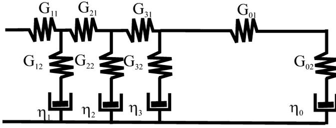
Fig. 4. The chain of Burgers elements; the completed Mervin model of the solid elastic network plunged in a fluid.
