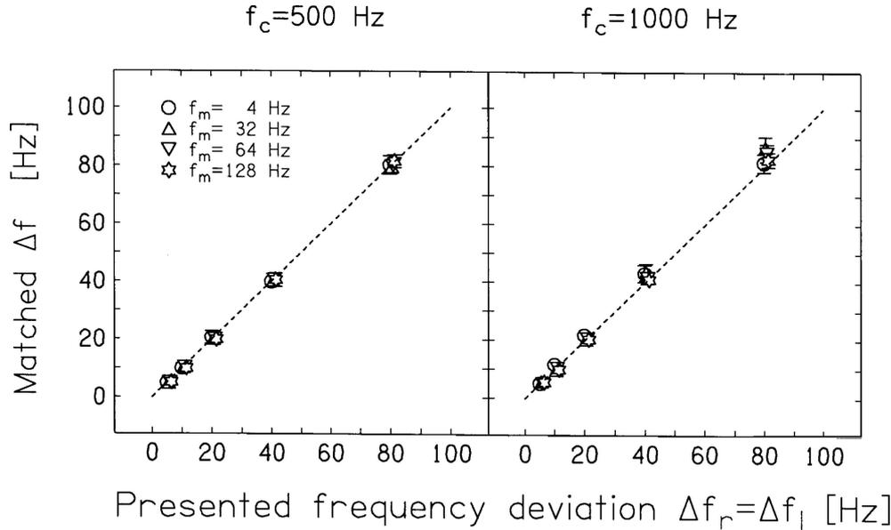
Fig. 5. Dependence of the binaurally perceived frequency deviation ( $\Delta f$ ) on the frequency deviation presented to the left ( $\Delta f_l$ ) and right ( $\Delta f_r$ ) ear, under conditions of diotic presentation ( $\Delta f_l = \Delta f_r$ ). The frequency of carrier signals equal 500 and 1000 Hz. The modulating frequency is the parameter of the data. Data averaged across three subjects.
