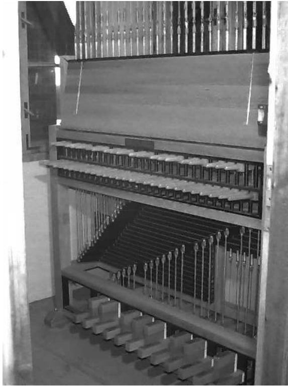
Fig. 2. St. Catherine's carillon keyboard (the chromatic scale of 49 keys and the transmission rods are well visible, the pedal keys are suspended below).
