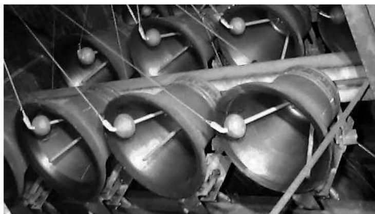
Fig. 4. Carillon bells equipped with a new mechanical system of clappers and pull wires (electromagnetic outer hammers are also visible).
