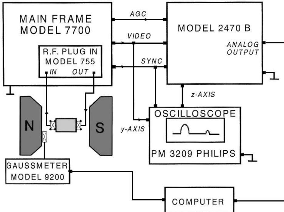
Fig. 1. A block diagram of the measuring system.
