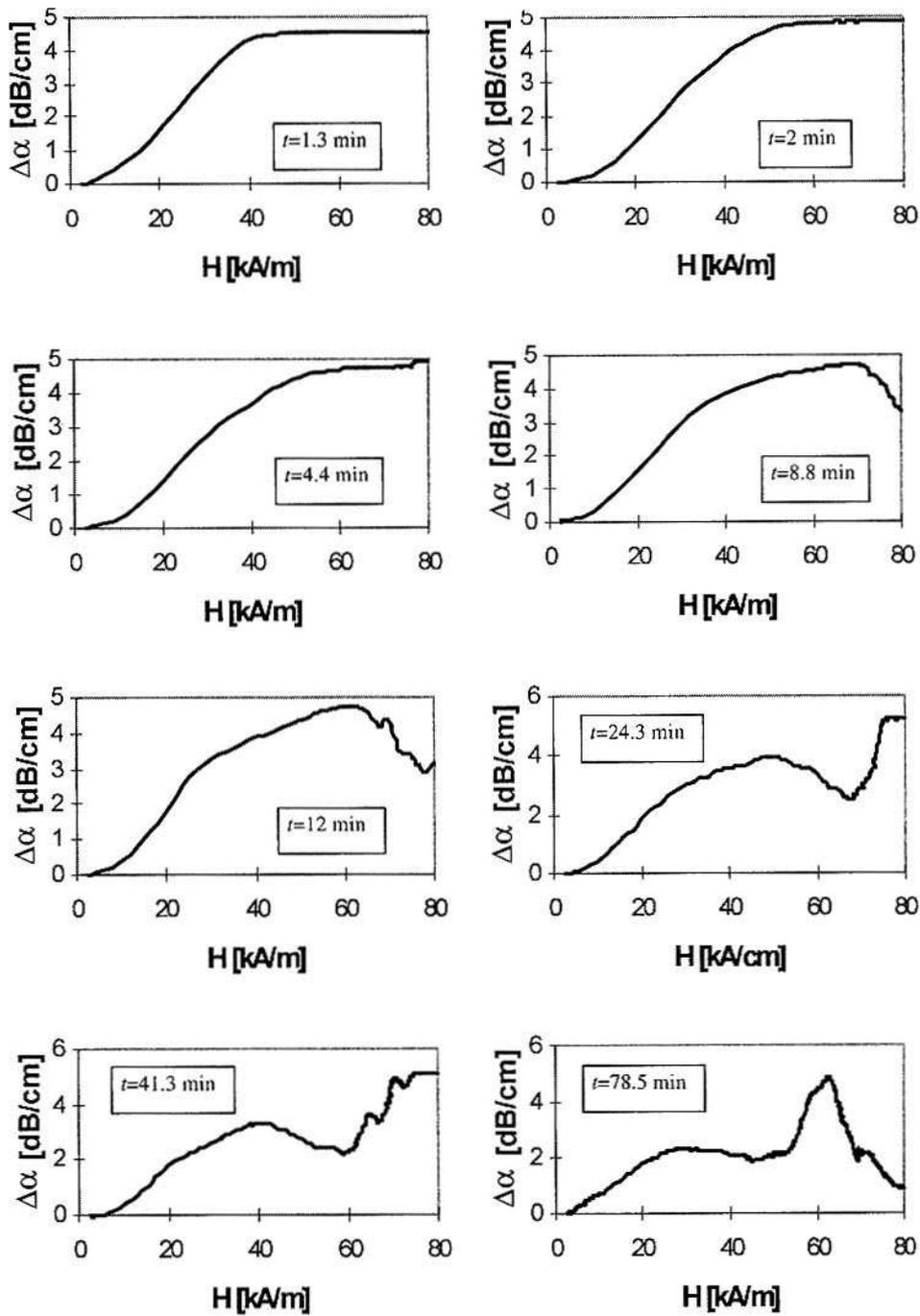
Fig. 3. Dependence of changes  $\Delta\alpha$  of ultrasonic wave of the frequency  $f = 6.12$  MHz as a function of magnetic field intensity  $H$ , where  $H \parallel k$ .
