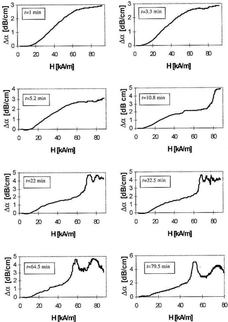
Fig. 5. Dependence of changes  $\Delta\alpha$  of ultrasonic wave of the frequency  $f = 6.12$  MHz as a function of magnetic field intensity  $H$  where  $H \perp k$ .
