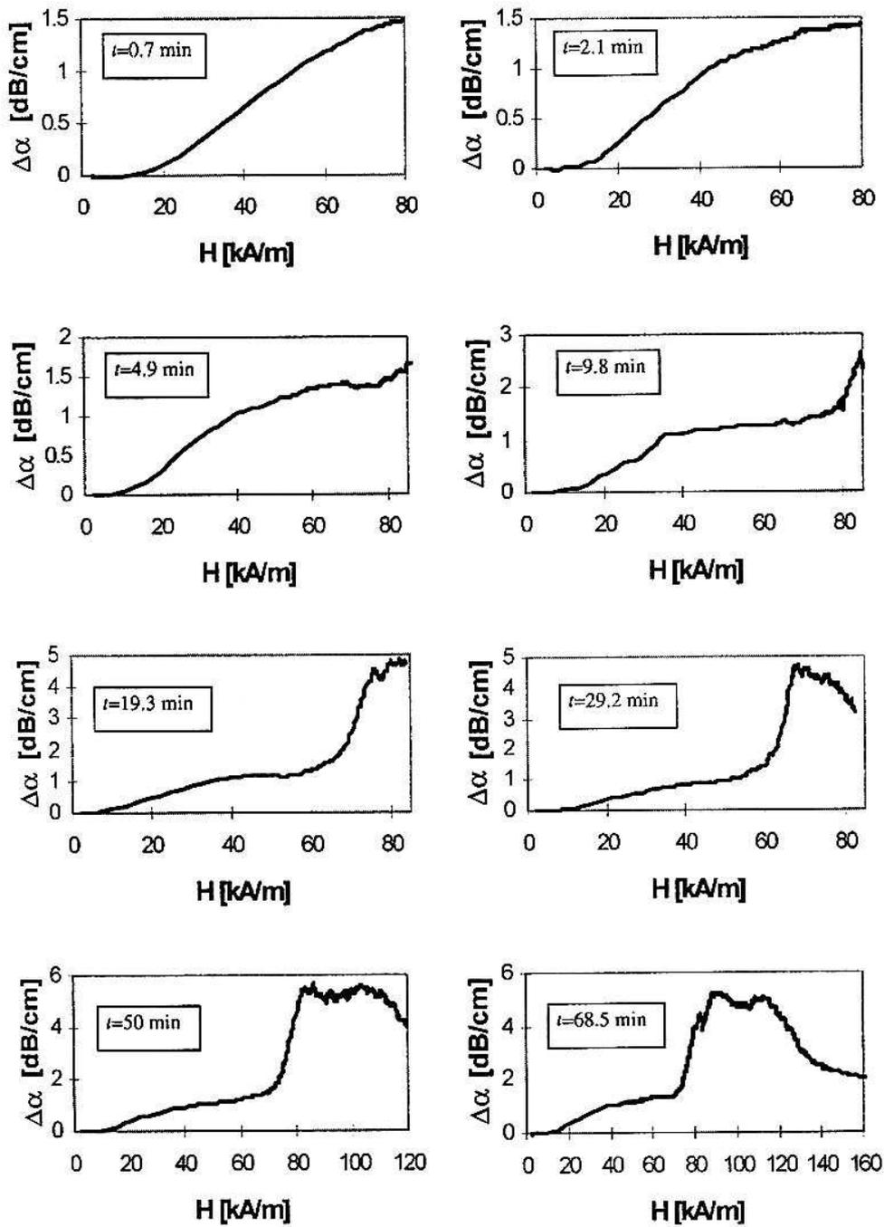
Fig. 4. Dependence of changes  $\Delta\alpha$  of ultrasonic wave of the frequency  $f = 3.6$  MHz as a function of magnetic field intensity  $H$  where  $H \perp k$ .
