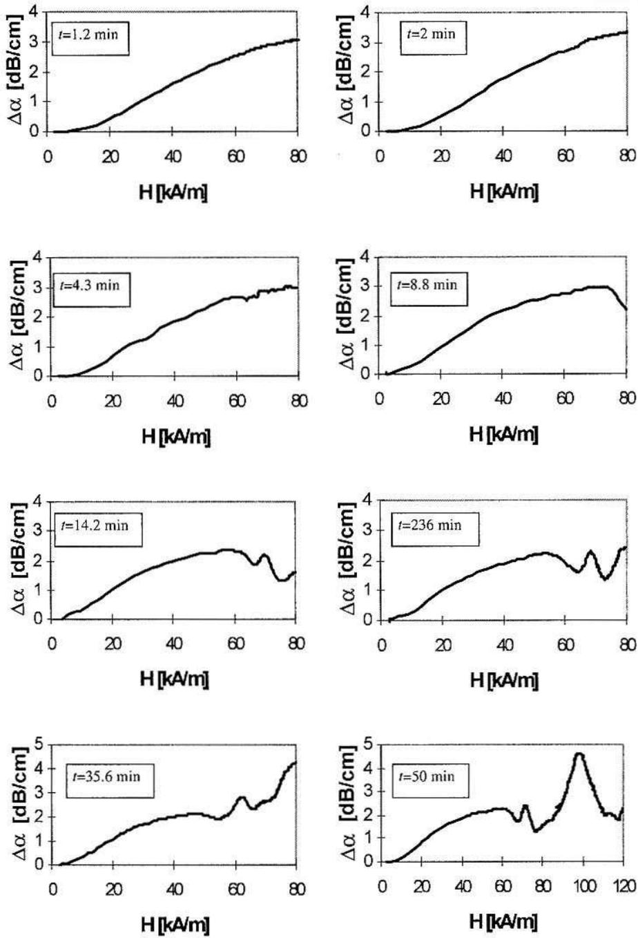
Fig. 2. Dependence of changes  $\Delta\alpha$  of ultrasonic wave of the frequency  $f = 3.6$  MHz as a function of magnetic field intensity  $H$ , where  $H \parallel k$ .
