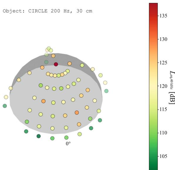
Fig. 11. Visualization of the results of ultrasonic noise tests at selected points of the hemisphere for an object in the form of a circle at a height of 30 cm ( $r = 2$  cm, modulation frequency 200 Hz).
