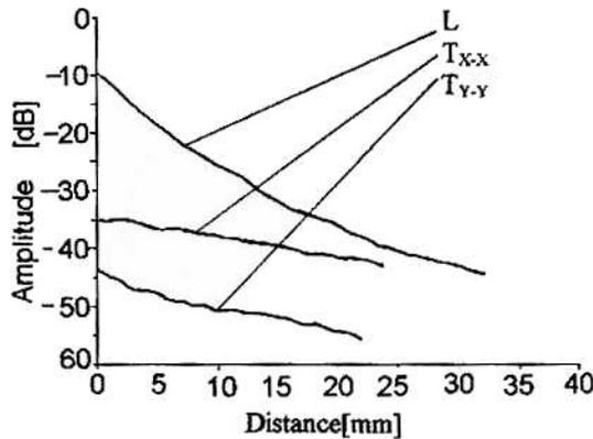
Fig. 2. Comparison of amplitude distribution of longitudinal (curve-L)- and shear (curves  $T_{X-X}$ ,  $T_{Y-Y}$ ) in one plane X-Z,  $y = 0$ ) waves versus distance from the epicenter in the PVC plate, probe 2.25 MHz;  $T_{X-X}$ -direction of polarization X-X,  $T_{Y-Y}$ -direction of polarization Y-Y.
