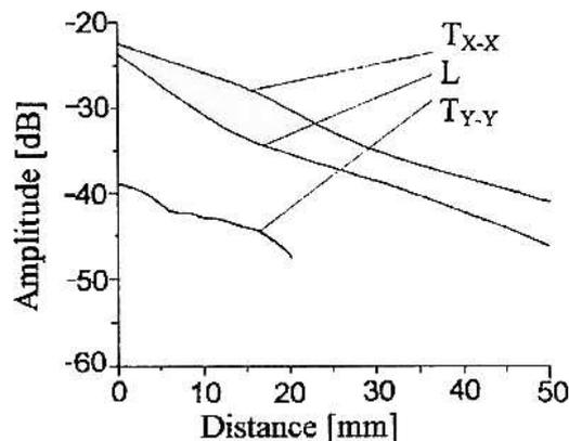
Fig. 3. Comparison of amplitudes of longitudinal (curve-L)- and shear (curves  $T_{X-X}$ ,  $T_{Y-Y}$ ) — wave distribution versus distance from epicenter, probe 2.25 MHz coupled on edge in PVC plate;  $T_{X-X}$ -direction of polarization X–X,  $T_{Y-Y}$ -direction of polarization Y–Y.
