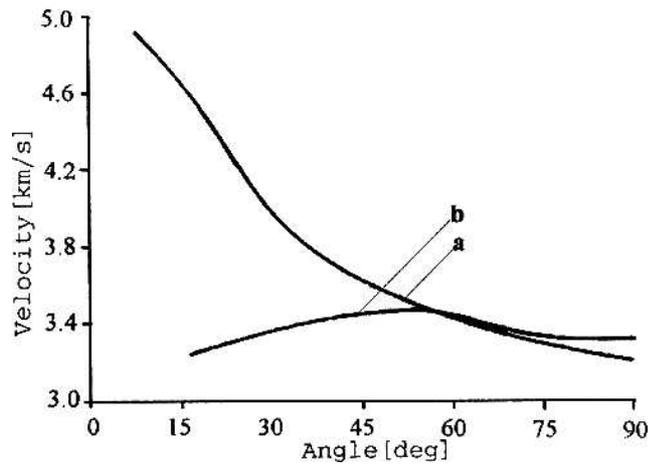
Fig. 7. Velocity of the longitudinal pulse in a GFC plate measured with a 2.25 MHz transducer. Curve a — measurement in the X-Z plane, curve b — measurement in the Y-Z plane.
