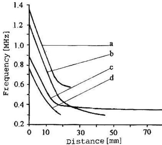
Fig. 9. Frequency distribution of a longitudinal wave: in a GFC plate with free surface measured in the direction perpendicular to fibres (curve a) or in the fibre direction (curve b); and in a GFC plate with constrained surface measured in the fibre direction (curve c) or in the direction perpendicular to the fibres (curve d).
