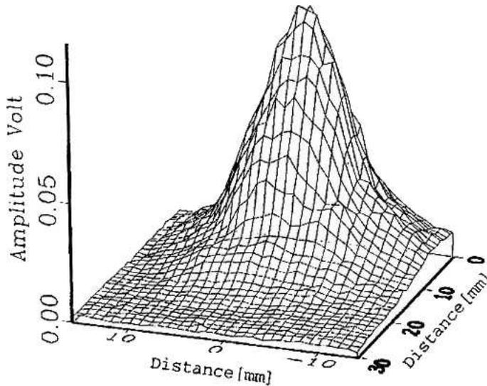
Fig. 6. The 3-D amplitude distribution of a longitudinal wave in the GFC cuboid measured with a 2.25 MHz transducer.
