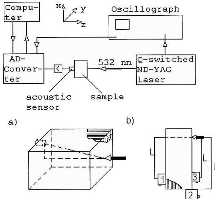
Fig. 1. Measuring stand with Nd:YAG laser; a) measurements in GFK-cuboid; b) measurement in GFK- or PVC-plate.
