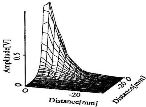
Fig. 4. The 3-D amplitude distribution of a longitudinal wave in the PVC plate measured by the 2.25 MHz probe.
