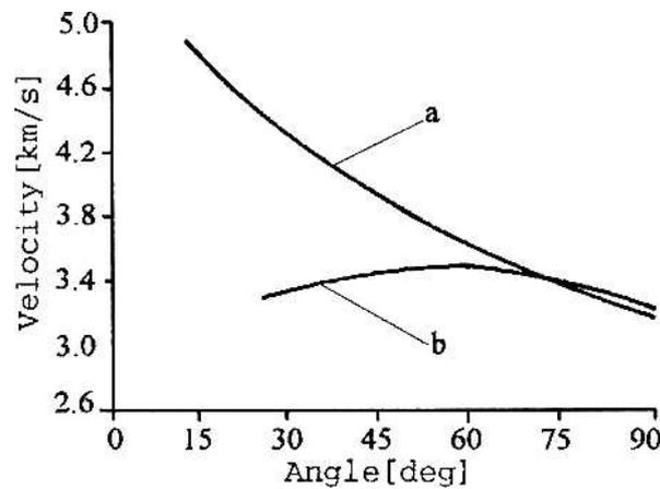
Fig. 8. Velocity of a longitudinal pulse in a GFC plate measured with an AE-transducer. Curve a — measurement in the X-Z plane, curve b — measurement in the Y-Z plane.
