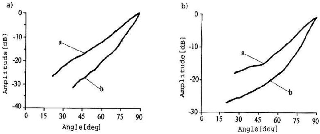
Fig. 5. 1-D amplitude distribution in a GFC plate; a) measurements perpendicular to fibres b) measurements in the fibre direction; a — curve measured with an AE-transducer, b — curve measured with a 2.25 MHz transducer.
