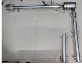
Fig. 5. Experimental setup for TL measurement of the fabricated mufflers.
