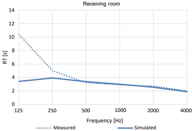
Fig. 11. RT measured and simulated in CATT-Acoustic software in the large receiving reverberation room. The simulation parameters were as follows: 50 000 rays, model 1, consideration of air sound absorption, ray tracing for 4500 ms, three source positions and ten microphone positions.
