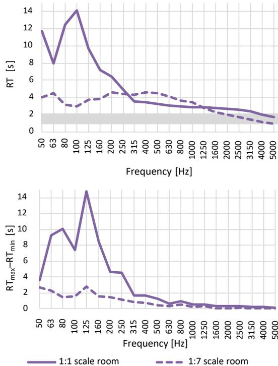
Fig. 14. RT and the scatter of the results between individual measurement points in the full-size receiving room (1:1 scale room) and its 1:7 scale equivalent. In the RT diagram, the grey colour indicates the RT ranges recommended by ISO (2021c) standard.
