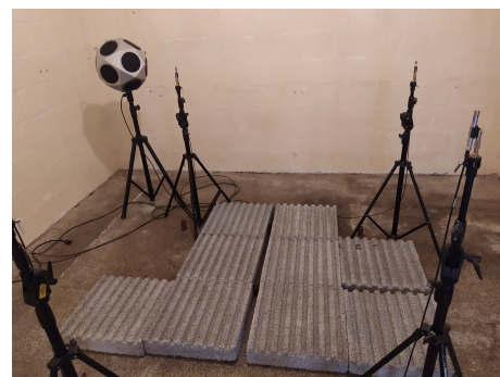
Fig. 6. Test setup in the reverberation chamber.
