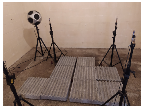
Fig. 6. Test setup in the reverberation chamber.
