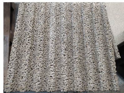
Fig. 1. Sound absorbing panels with dimensions 500\text{ mm} \times 500\text{ mm} \times 100\text{ mm} .
