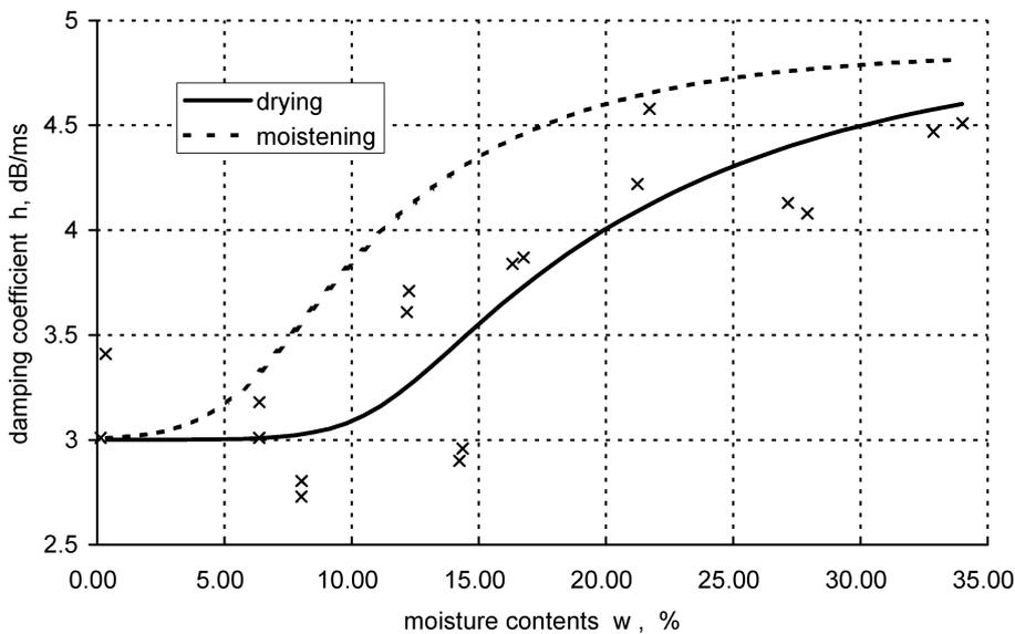
Fig. 7. Change of the damping coefficient in the oak wood log during drying process versus moisture content for vibrations in the direction perpendicular to the layers of fibres; Approaching curve:  $h = 4.85 - 1.85(8e^{0.7(w-14)} + 1)^{-1/8}$ .
