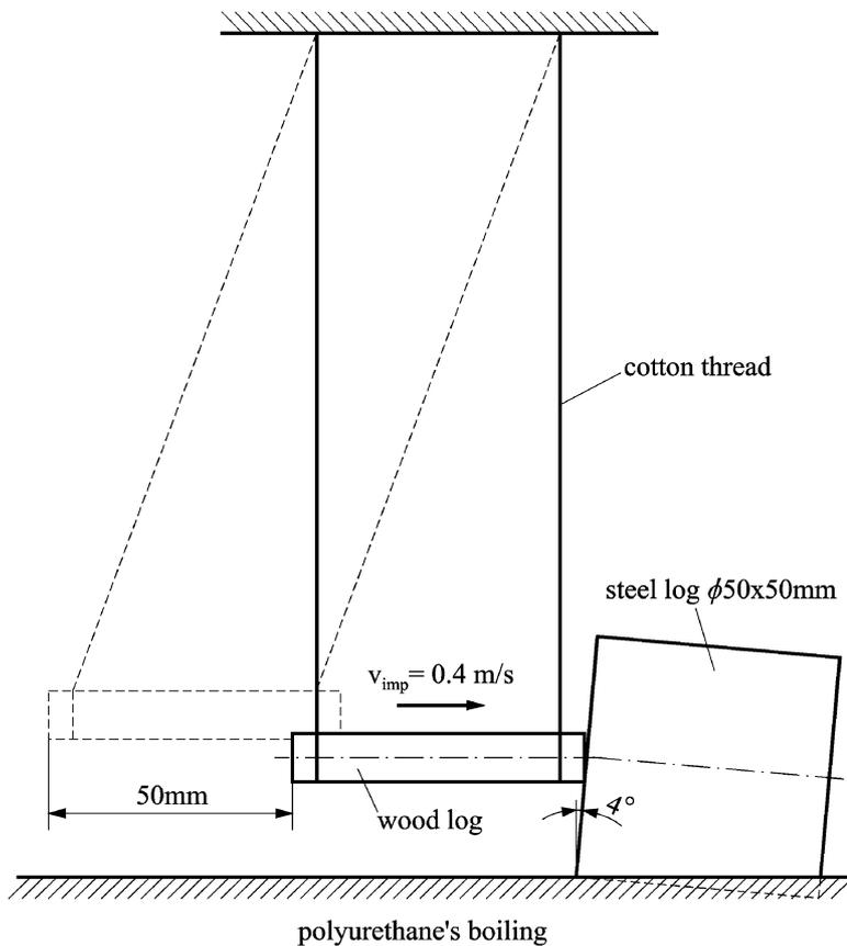
Fig. 2. Scheme of the stand for investigations of the influence of moisture contents in oak wood on the damping of its free vibrations.
