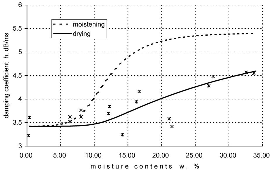
Fig. 9. Change of the damping coefficient in the oak wood log during drying process versus moisture content for vibrations in the direction parallel to the layers of fibres;
