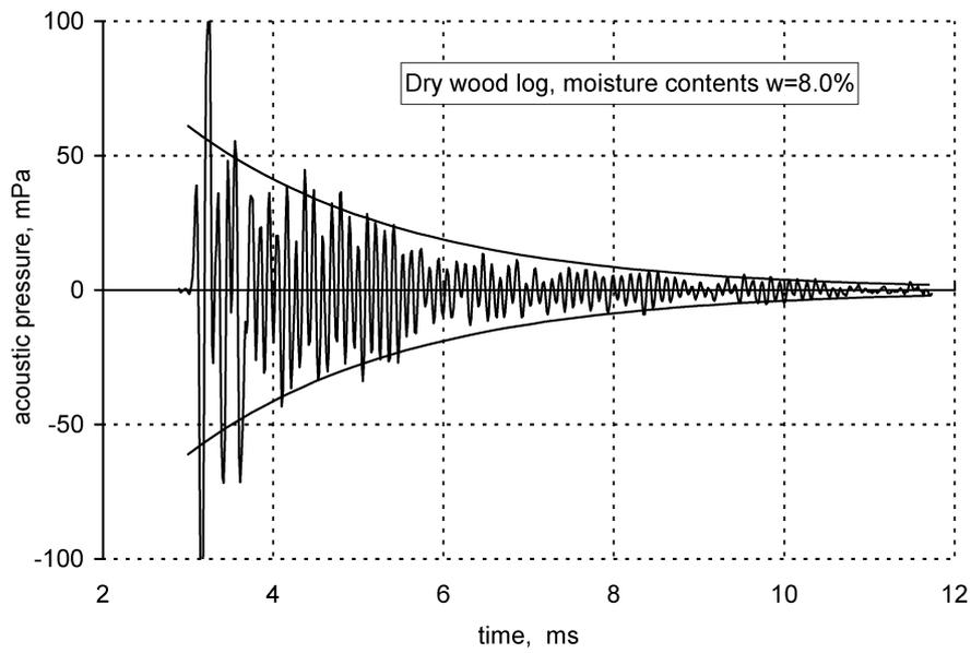
Fig. 4. Decreasing acoustic pressure, suitable to flexural free vibrations of the dry wood log in the direction perpendicular to the layers of its fibres, versus time; Envelope:  $|p| = 66.2 \cdot 10^{-3.60(t-3.125)/20}$ .
