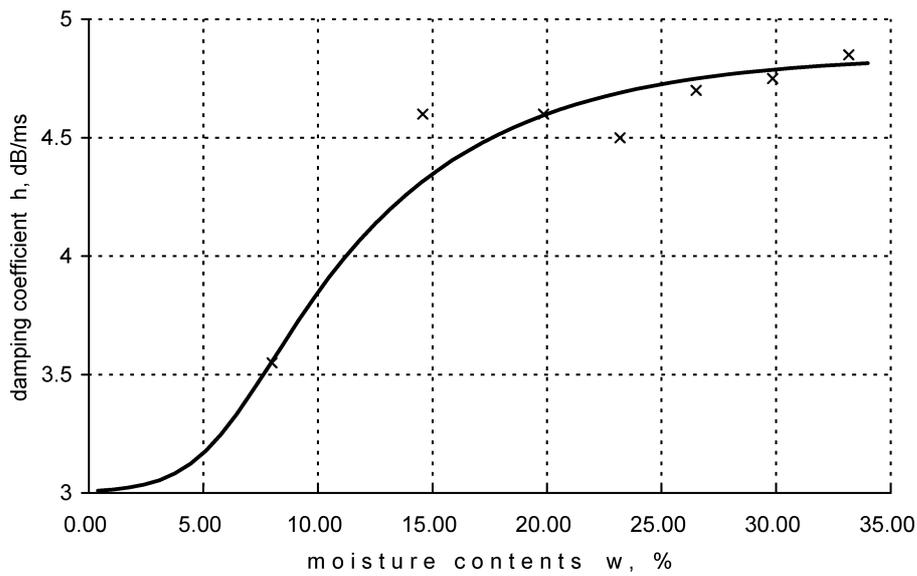
Fig. 6. Change of the damping coefficient in the oak wood log during moistening process versus moisture content for vibrations in the direction perpendicular to the layers of fibres; Approaching curve:  $h = 4.85 - 1.85(5e^{0.7(w-8)} + 1)^{-1/5}$ .
