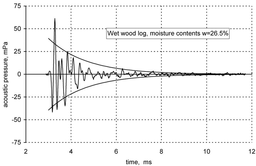
Fig. 5. Decreasing acoustic pressure, suitable to flexural free vibrations of the wet wood log in the direction perpendicular to the layers of its fibres versus time; Envelope:  $|p| = 25.1 \cdot 10^{-4.75(t-3.125)/20}$ .
