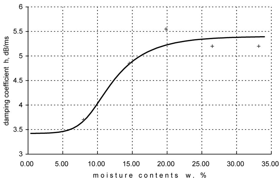
Fig. 8. Change of the damping coefficient in the oak wood log during moistening process versus moisture content for vibrations in the direction parallel to the layers of fibres;
