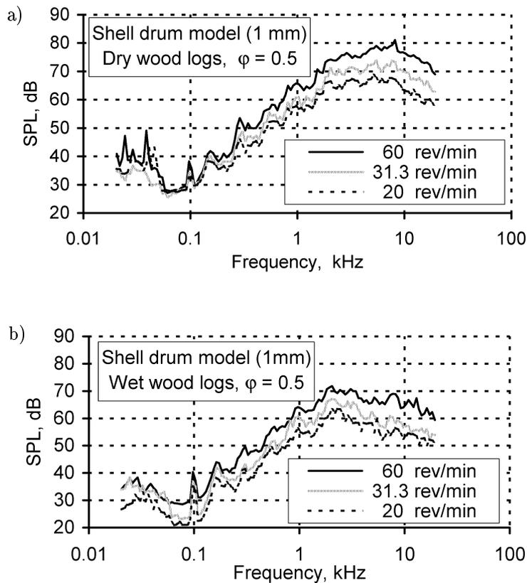
Fig. 1. Noise spectra of the drum model made of a cylindrical steel shell (1 mm thick) at rotational speeds: 20, 31.3, 60 rev/min; a) filled up with dry wood logs; b) filled up with wet wood logs. Fulfilment degree  $\varphi = 0.5$ .
