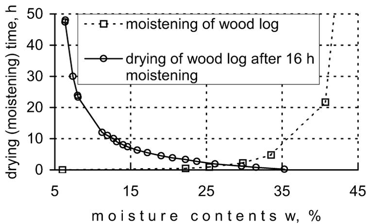
Fig. 3. Dependence of the moisture contents (in %) on time (in hours) of the tested wood log in the moistening and/or drying process.
