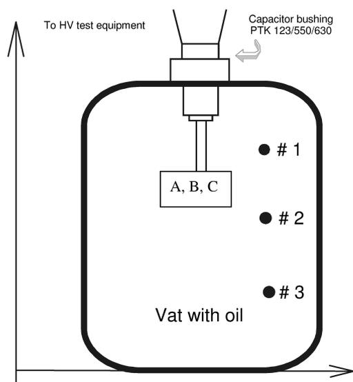
Fig. 2. Set of elements for the testing of partial discharges: — vat with oil, — bushing with different endings A, B, C — acoustic emission measuring system AE COMP-DEMA, — HV test equipment (supply voltage, ERA system).
