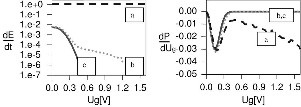
Fig. 10. The amplitude distributions of power of AE signal  $dE/dt$  and the first derivative of the amplitude distributions of power of AE signal  $dP/dU_g$  versus the discrimination threshold level  $U_g$  in the following measuring situations: a) PD source modeled with C,  $U = 90$  kV,  $q > 1600$  pC, 50 dB, b) PD source modeled with C,  $U = 85$  kV,  $q = 200$  pC, 50 dB, c) PD source modeled with C,  $U = 74$  kV,  $q =$  a few pC, 50 dB.
