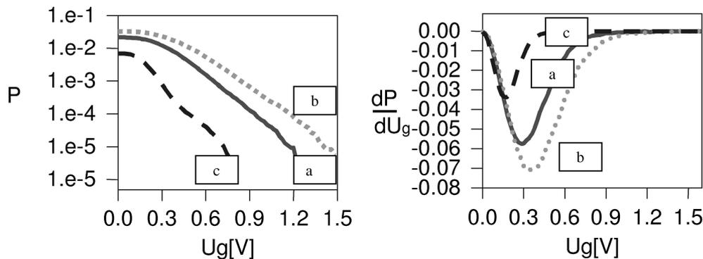
Fig. 9. The amplitude distributions of power of the AE signal  $P$  and the first derivative of the amplitude distributions of power of the AE signal  $dP/dU_g$  versus the discrimination threshold level  $U_g$  in the following measuring situations: a) PD source modeled with B,  $U = 123$  kV,  $q \gg 1600$  pC, 40 dB, b) PD source modeled with B,  $U = 106$  kV,  $q = 560$  pC, 50 dB, c) PD source modeled with B,  $U = 90$  kV,  $q = 36$  pC, 50 dB.
