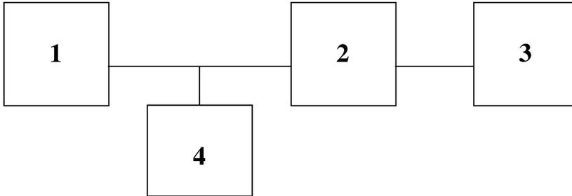
Fig. 1. Block scheme of the AE measuring system called COMP-DEMA: 1 — set of DEMA instruments, 2 — CB6-TP measuring terminal and PCI-610E measuring card, 3 — PCIII portable PFX-12, 4 — oscilloscope.
