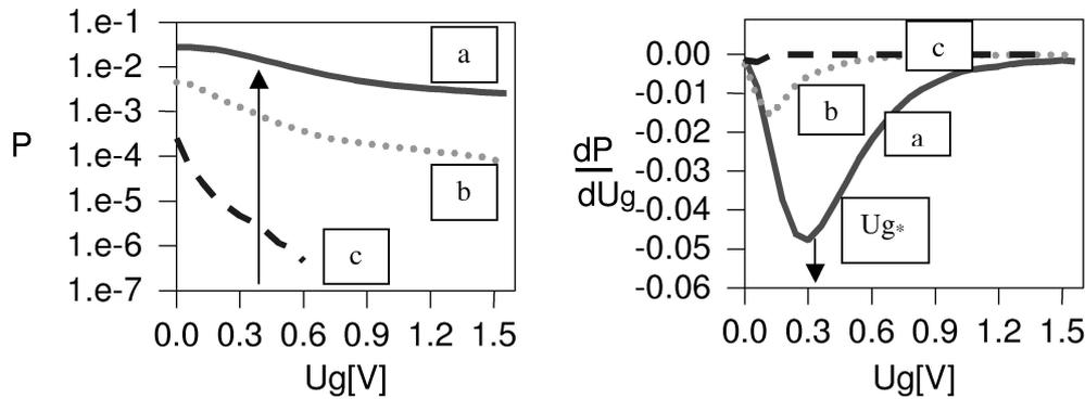
Fig. 8. The amplitude distributions of power of the AE signal  $P$  and the first derivative of the amplitude distributions of power of the AE signal  $dP/dU_g$  versus the discrimination threshold level  $U_g$  in the following measuring situations: a) PD source modeled with A,  $U = 123$  kV;  $q \gg 1600$  pC, 30 dB, b) PD source modeled with A,  $U = 106$  kV;  $q \gg 1600$  pC, 30 dB, c) PD source modeled with A,  $U = 74$  kV;  $q \gg 1600$  pC, 30 dB.
