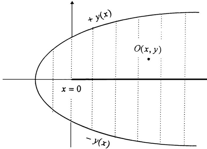
Fig. 4. The cut-off lines,  $\pm y(x)$  (Eq. (21)), and the ground track,  $y = 0$  with  $x > 0$ , for climbing or descending.
