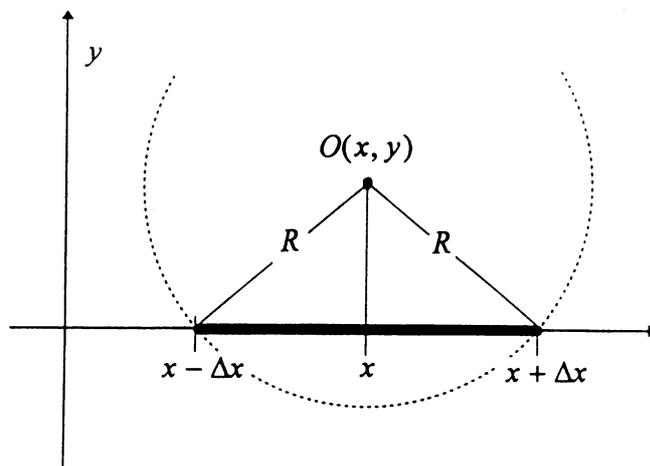
Fig. 2. Noise reaches the receiver,  $O(x, y)$ , when an aircraft is within a circle of radius  $R$  (Eq. (8)).
