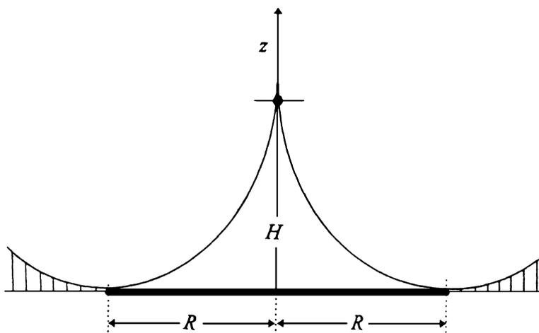
Fig. 1. Shadow zone caused by the upward refracted rays.
