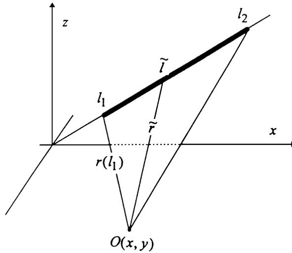
Fig. 5. Noise-producing path segment  $(l_1, l_2)$  (Eq. (22)), with the shortest distance,  $r(l_1)$  (Eq. (25)).
