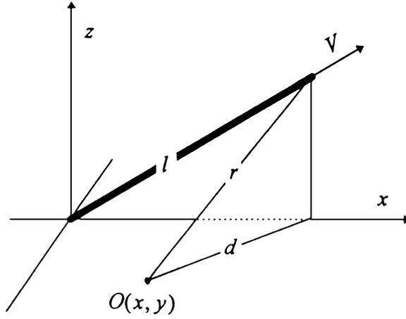
Fig. 3. The instantaneous location of an aircraft is determined by the length of climbing path,  $l$ , and the climbing angle,  $\delta$ .
