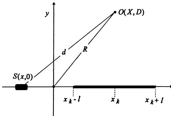
Fig. 3. Distance  $d$  between the receiver  $O$  and the vehicle  $S$  (Eq. (8)) and the distance  $R$  between the receiver and the center of the stopping line (Eq. (35)).
