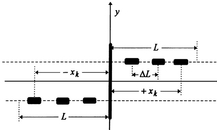
Fig. 1. Queues of waiting vehicles with the average length,  $L$ , the same on both sides of the stopping line.
