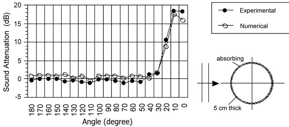
Fig. 9. Sound attenuation and scattering from an absorbing cylinder:  $kR = 18.3$ ; distance from a point in the field to the center of the cylinder: 132 cm, number of monopoles:  $N = 73$ , surface impedance:  $Z = 267.3 + j 92.8$ .
