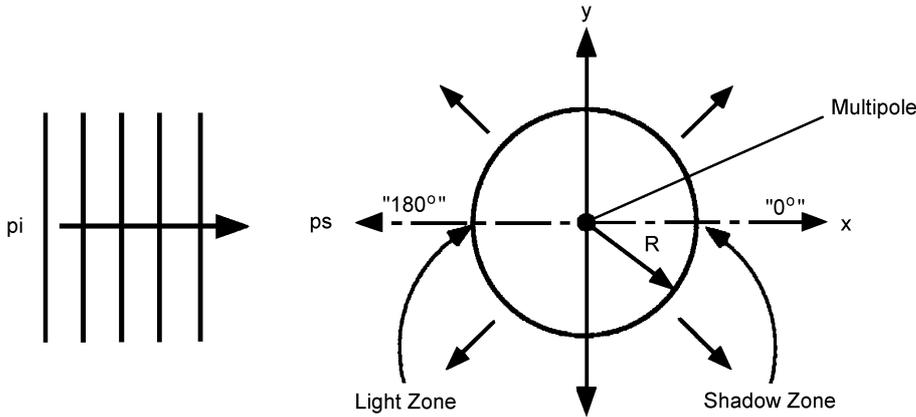
Fig. 2. One-point multipole method for the rigid and absorbing circular cylinder.
