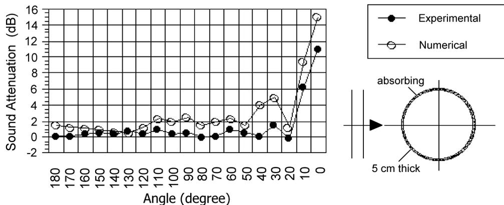
Fig. 8. Sound attenuation and scattering from an absorbing cylinder:  $kR = 14.65$ ; distance from a point in the field to the center of the cylinder: 130 cm, number of monopoles:  $N = 59$ , surface impedance:  $Z = 250.3 - j 200$ .
