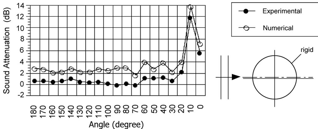
Fig. 7. Sound attenuation and scattering from a rigid cylinder:  $kR = 13.7$ ; distance from a point in the field to the center of the cylinder: 47 cm, number of monopoles:  $N = 55$ .
