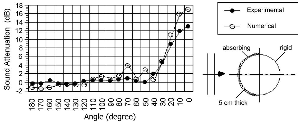
Fig. 10. Sound attenuation and scattering from a half-absorbing and half-rigid cylinder:  $kR = 14.65$ ; distance from a point in the field to the center of the cylinder: 47 cm, number of monopoles:  $N = 59$ , surface impedance:  $Z = 250.3 - j 200$ .
