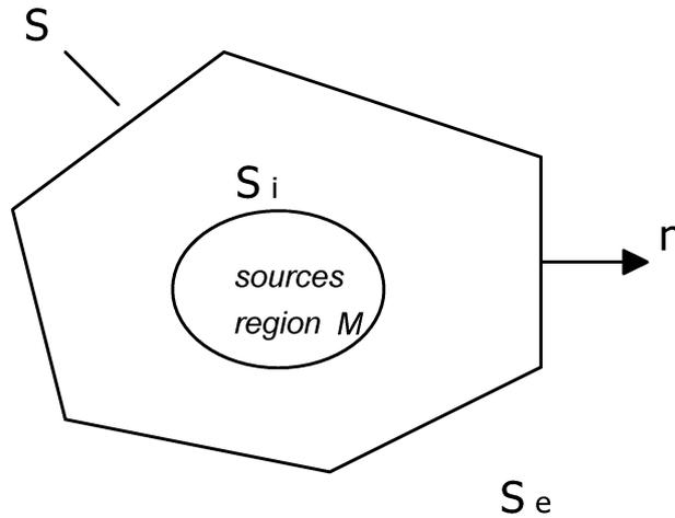
Fig. 1. Geometry of the radiation and scattering problem (OCHMANN [12]).
