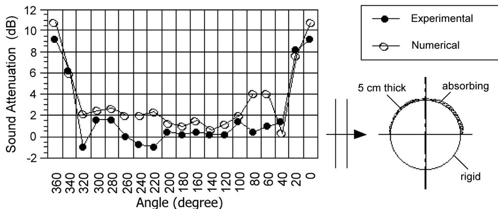
Fig. 11. Sound attenuation and scattering for a mixed case:  $kR = 9.16$ ; distance from a point in the field to the center of the cylinder: 47 cm, number of monopoles:  $N = 37$ , surface impedance:  $Z = 564 + j 542.3$ .
