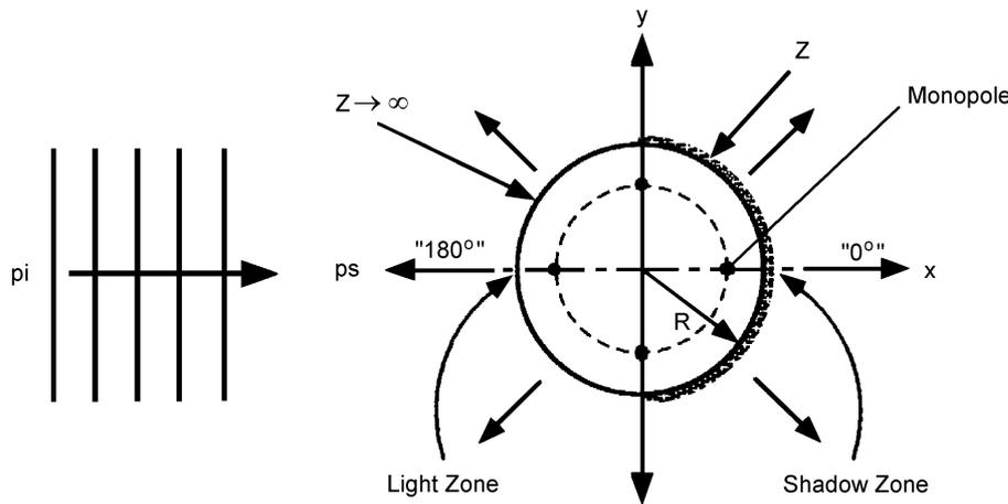
Fig. 3. Single Layer Method for the rigid and absorbing circular cylinder.
