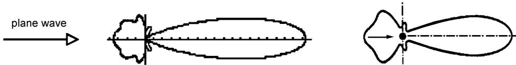
Fig. 6. Comparison between the calculation of sound scattering with the source simulation technique and the analytical solution for  $\lambda = (2/5)\pi R$ .
