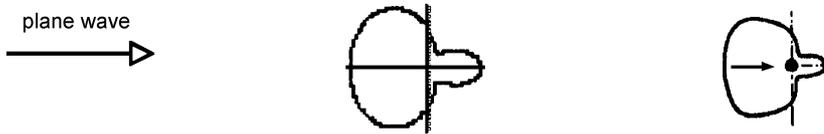
Fig. 5. Comparison between the calculation of sound scattering with the source simulation technique and the analytical solution for  $\lambda = 2\pi R$ .
