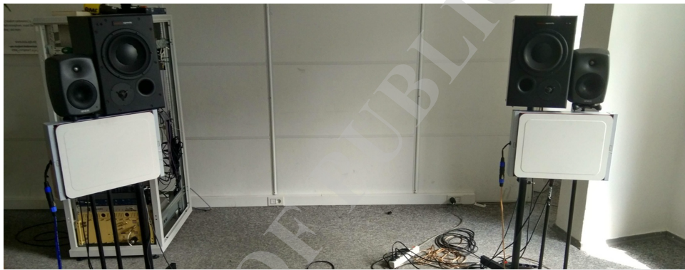
Figure 1. Exemplary arrangement of loudspeakers. During the experiment, loudspeakers were hidden behind an acoustically transparent curtain.
