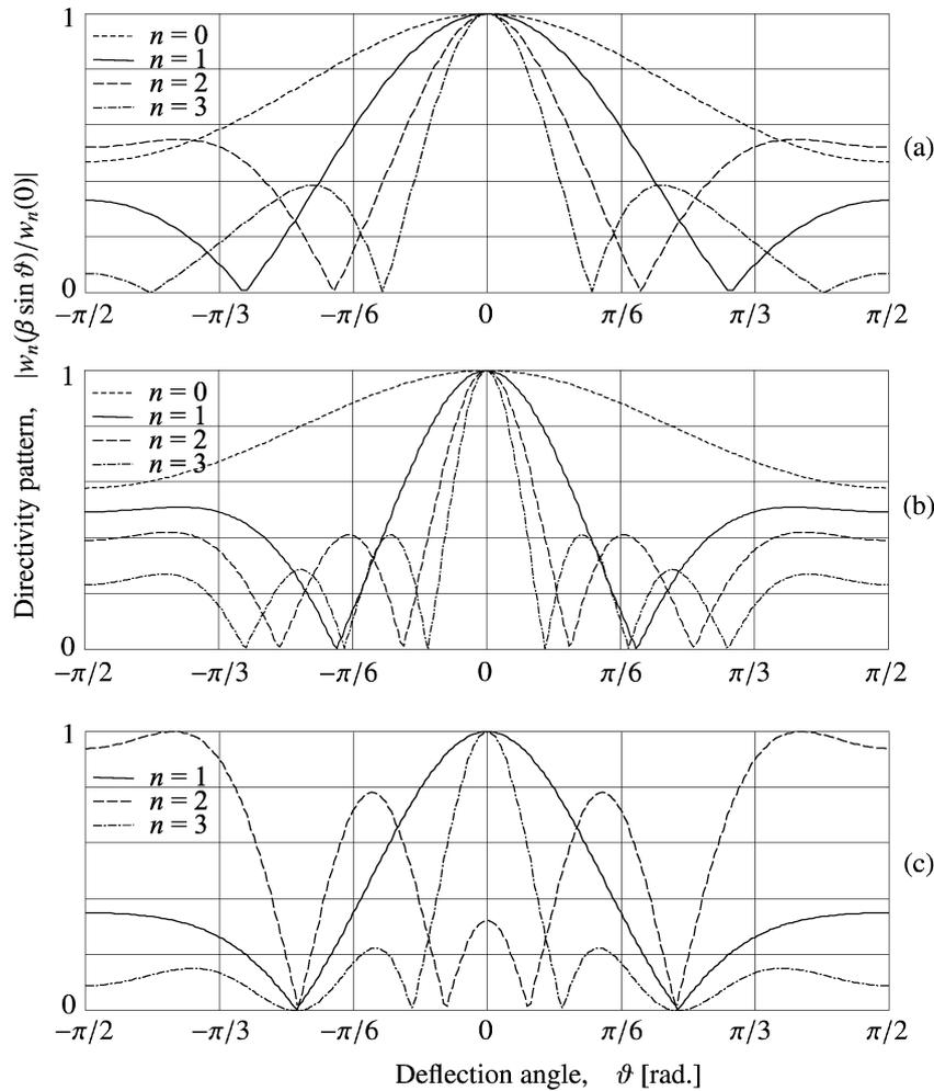
Fig. 2. The directivity pattern of the sound radiation  $|w_n(\beta \sin \vartheta)/w_n(0)|$  of an annular plate for  $r_2/r_1 = 2$  and for the value  $x_n/2$  of the dimensionless wavenumber  $\beta$  with the following edge configurations: (a) clamped-free, (b) free-clamped, (c) clamped-clamped, (cf., reference [14]).
