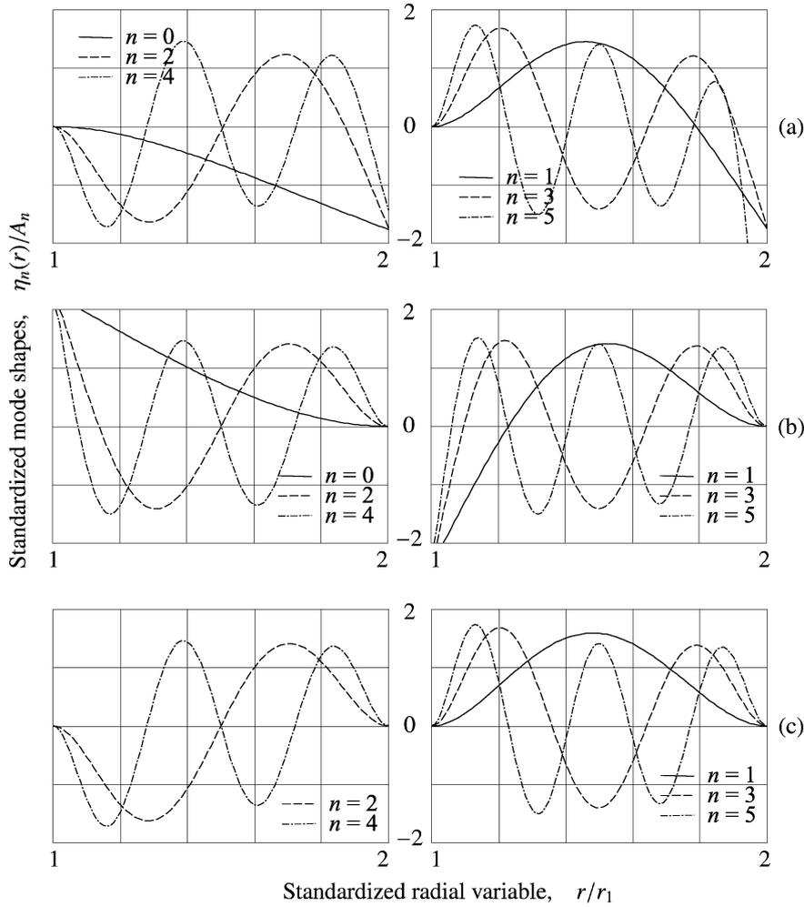
Fig. 1. The values of standardized mode shapes  $\eta_n(r)/A_n$  of an annular plate for  $r_2/r_1 = 2$  valid for the following edge configurations: (a) clamped-free, (b) free-clamped, (c) clamped-clamped, (cf. references [17, 18, 20, 24]).
