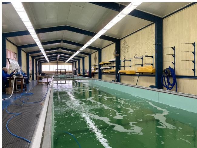
Fig. 3. Hydrodynamic testing channel.
