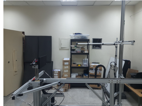
Fig. 1. Klippel GmbH near-field scanner measurement setup.
