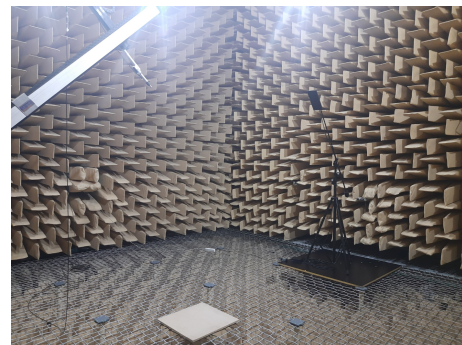
Fig. 2. Directivity of reflected sound, measurement setup in an anechoic chamber.
