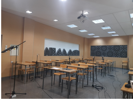
Fig. 6. Experimental setup for measuring reflections from the angled ceiling in the classroom.
