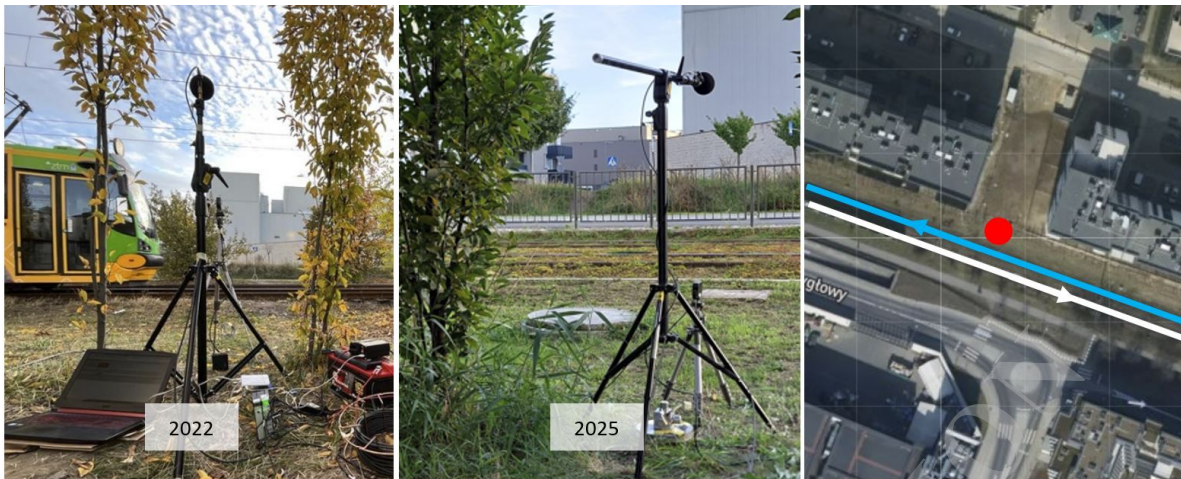
Figure 3: Pass-by noise measurement point: 2022 campaign (left) and 2025 campaign (centre) photos by the authors; satellite view (right) from the OpenAerialMap viewer (OpenAerialMap, 2026).
