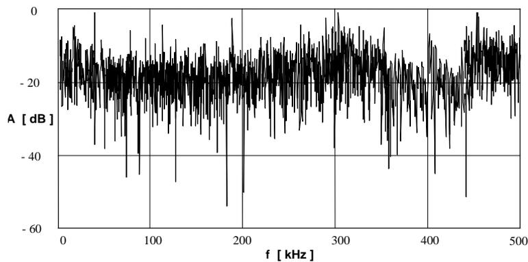
Fig. 8. Amplitude spectrum of a series of AE pulses generated by PD in oil in the “spike-plate” system during the positive voltage half-cycle ( $1^\circ$ ,  $\phi$  0.06 mm).
