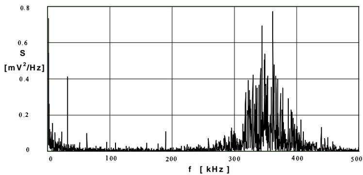
Fig. 15. Energy density spectrum of a series of AE pulses generated by PD in oil in the “spike-plate” system during the negative voltage half-cycle ( $22^\circ$ ,  $\phi$  0.6 mm).
