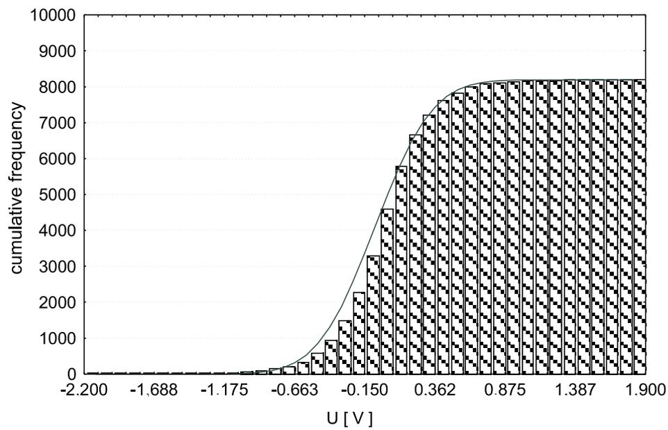
Fig. 2. Cumulative density function determined for the AE pulses generated by PDs of the multipoint-plane type at the positive voltage polarization.
