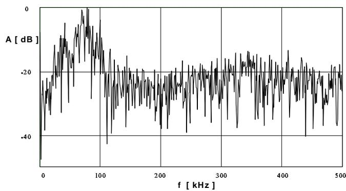
Fig. 6. Amplitude spectrum run for AE pulse series generated by in indeterminate-potential particles moving in oil, in the positive voltage half-period.
