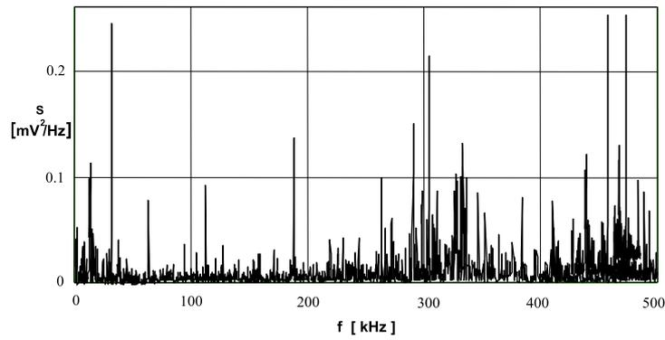
Fig. 10. Energy density spectrum of a series of AE pulses generated by PD in oil in the “spike-plate” system during the positive voltage half-cycle ( $1^\circ$ ,  $\phi$  0.06 mm).
