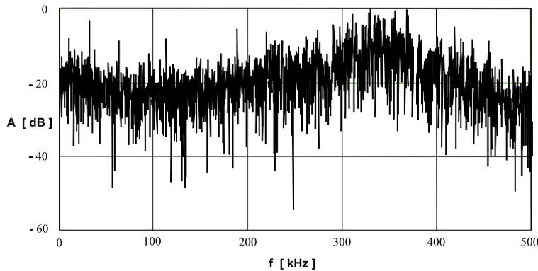
Fig. 9. Amplitude spectrum of a series of AE pulses generated by PD in oil in the “spike-plate” system during the negative voltage half-cycle ( $1^\circ$ ,  $\phi$  0.06 mm).
