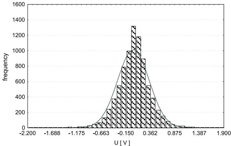
Fig. 1. Probability density functions (PDF) determined for the AE pulses generated by PDs of the multipoint-plane type at the positive voltage polarization.
