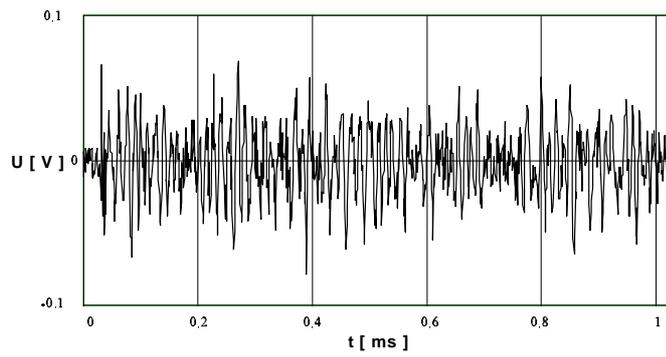
Fig. 5. Time run for AE pulse series generated by PDs in indeterminate-potential particles moving in oil, in the positive voltage half-period discharges.
