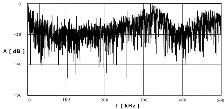
Fig. 12. Amplitude spectrum of a series of AE pulses generated by PD in oil in the “spike-plate” system during the positive voltage half-cycle ( $22^\circ$ ,  $\phi$  0.6 mm).
