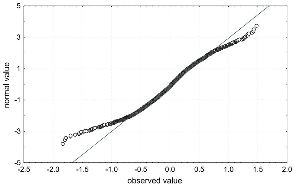
Fig. 3. Normal probability plot determined for the AE pulses generated by PDs of the multipoint-plane type at the positive voltage polarization.
