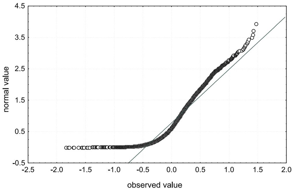
Fig. 4. Semi-normal probability plot determined for the AE pulses generated by PDs of the multipoint-plane type at the positive voltage polarization.
