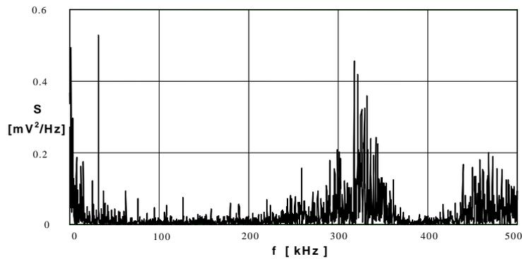
Fig. 14. Energy density spectrum of a series of AE pulses generated by PD in oil in the “spike-plate” system during the positive voltage half-cycle ( $22^\circ$ ,  $\phi$  0.6 mm).
