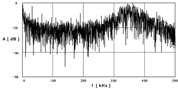
Fig. 13. Amplitude spectrum of a series of AE pulses generated by PD in oil in the “spike-plate” system during the negative voltage half-cycle ( $22^\circ$ ,  $\phi$  0.6 mm).
