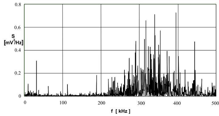
Fig. 11. Energy density spectrum of a series of AE pulses generated by PD in oil in the “spike-plate” system during the negative voltage half-cycle ( $1^\circ$ ,  $\phi$  0.06 mm).
