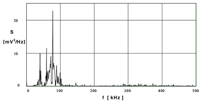
Fig. 7. Energy density spectrum run for AE pulse series generated by PDs in indeterminate-potential particles moving in oil, in the positive voltage half-period.
