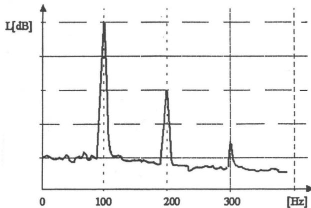
Fig. 18. Course of an acoustic pressure level  $L$  vs. frequency for typical power transformer operating at 50 Hz.
