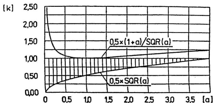
Fig. 2. The conditions for the phase compensation vs.  $x(t)$  and  $y(t)$  signal parameters.
