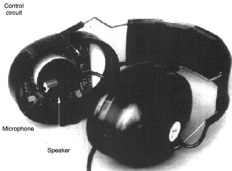
Fig. 16. The AOS-2 ear protector with active noise control system developed by CIOP-PIB.
