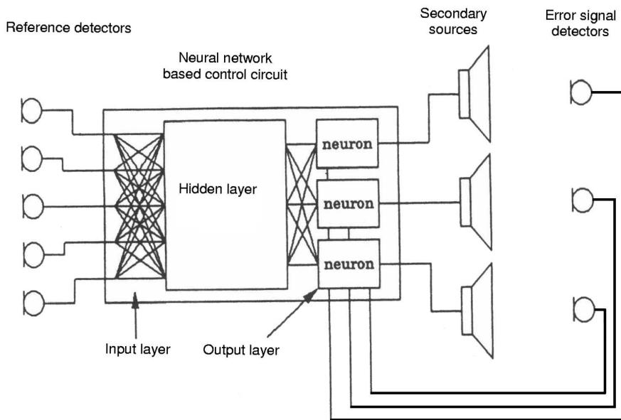
Fig. 21. The multi-channel active noise control system based on the neural network.
