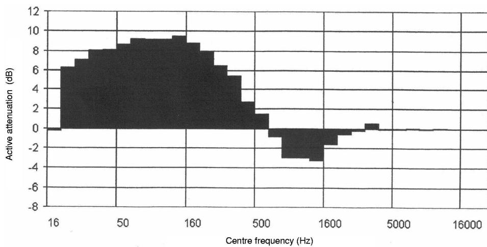
Fig. 17. Active noise attenuation for AOS-2 protector.
