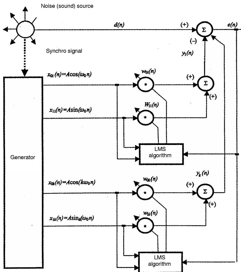
Fig. 13. Active noise control systems with two notch parallel filters.
