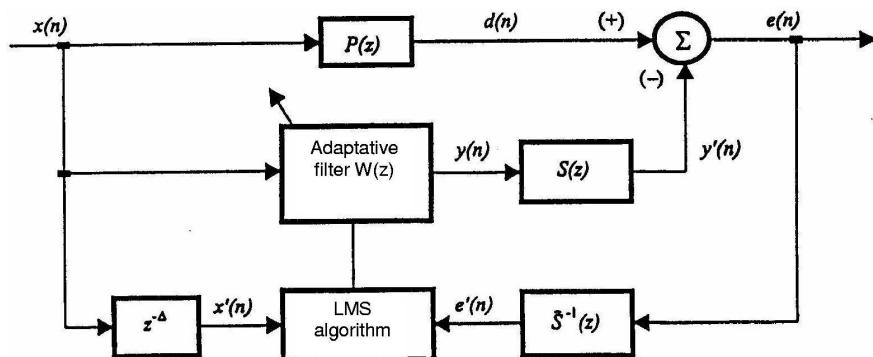
Fig. 12. The block diagram of the active noise control system incorporating the controller, which eliminates the secondary signal path effect.
