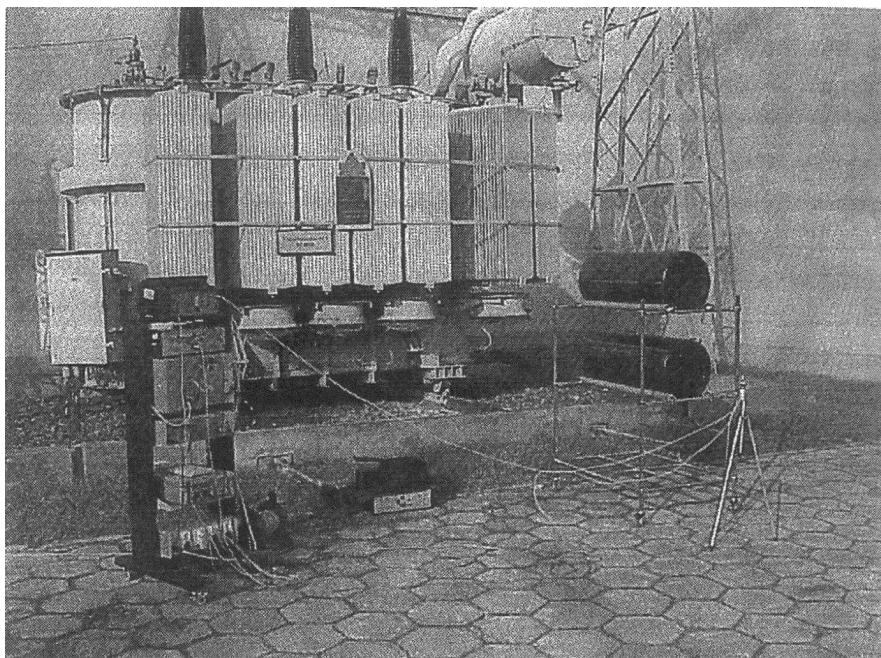
Fig. 20. The power transformer with the active noise control system implemented.
