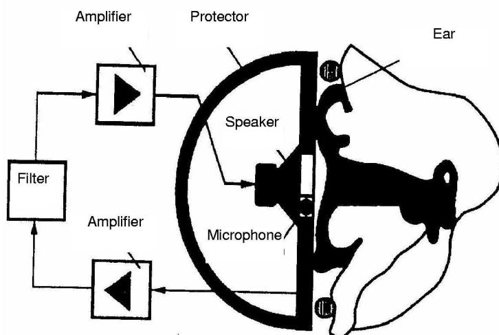
Fig. 15. The diagram of the ear protector with active noise control system.
