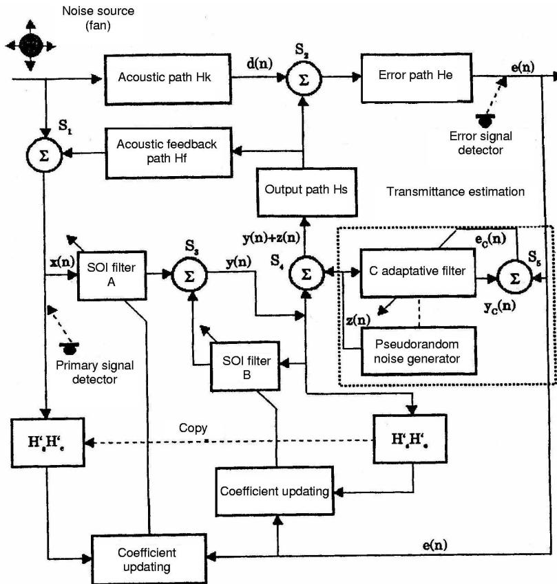
Fig. 8. Controller diagram.
