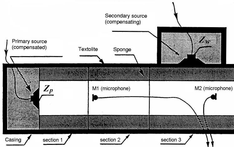
Fig. 6. Basic diagram of active noise control system in the waveguide.
