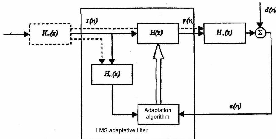
Fig. 11. The block diagram of LMS algorithm with filtered input.
