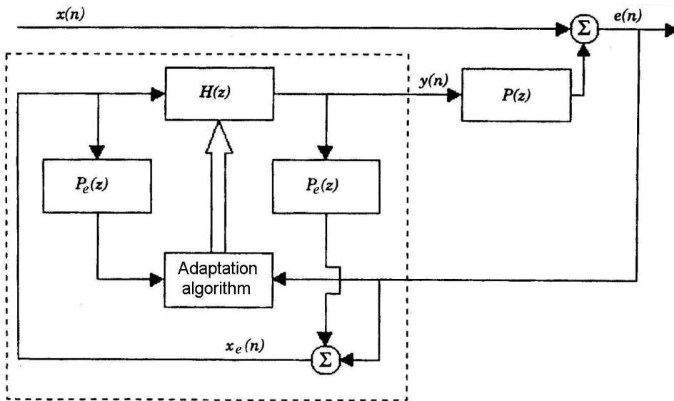
Fig. 9. The block diagram of the active noise control system with the controller and built-in reference model.
