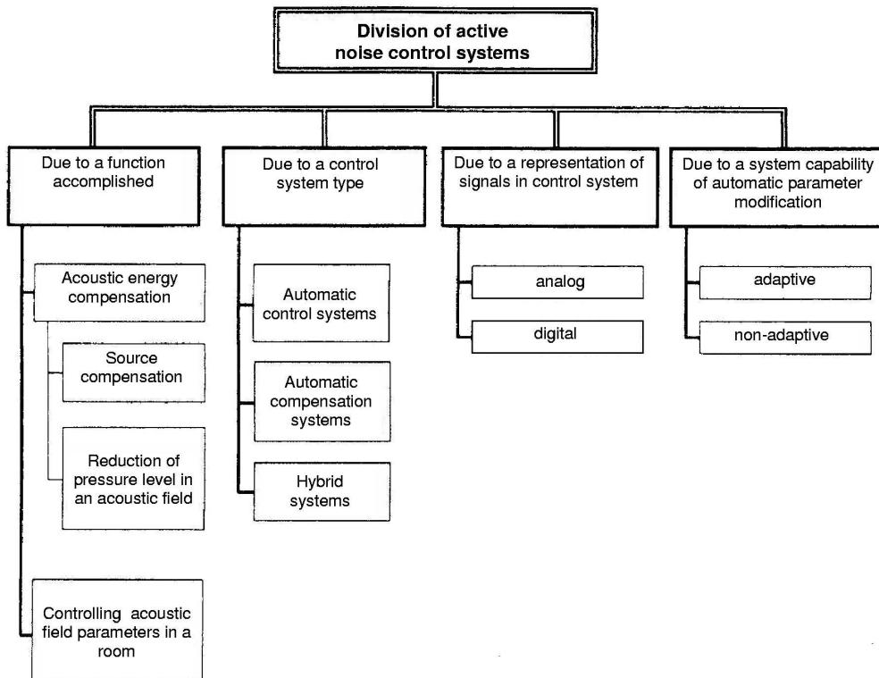
Fig. 5. Active noise control system classification.
