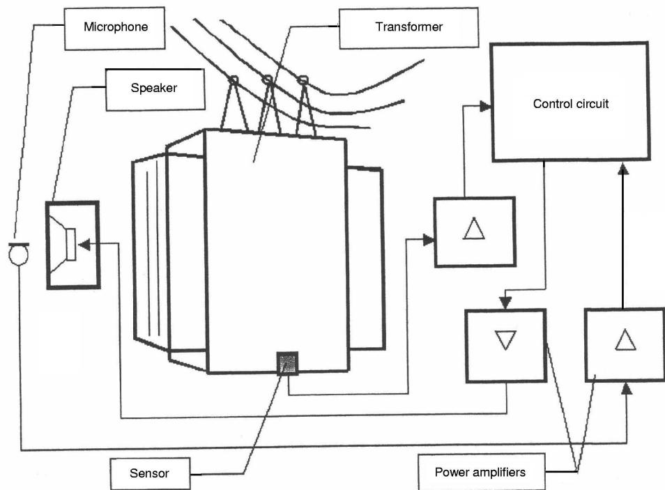
Fig. 19. The active noise control system for the power transformer.
