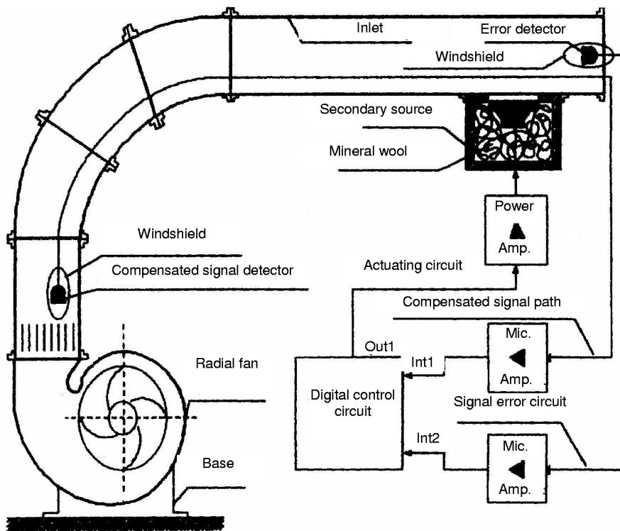
Fig. 14. The block diagram of active noise control system for the ventilation channel, developed and installed in CIOP-PIB.
