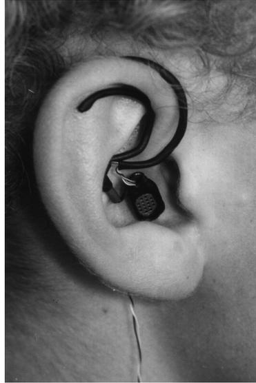
Fig. 7. Measuring microphone near the entrance of the hearing canal.
