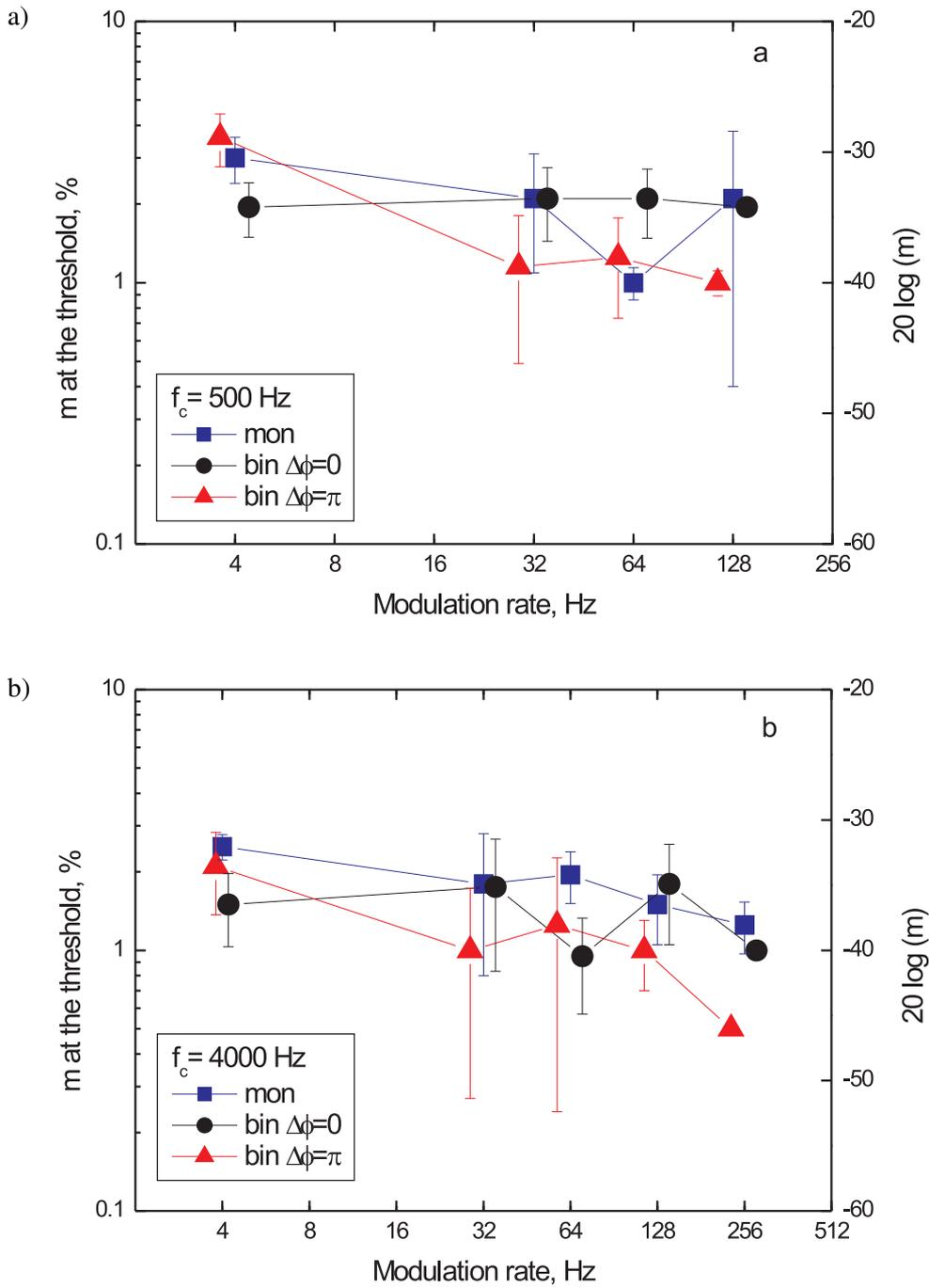
Fig. 1. Thresholds for amplitude modulation detection as a function of the modulation rate for a sinusoidal carrier at a frequency of 500 Hz (a) and 4000 Hz (b). The data present the mean thresholds for three subjects.
