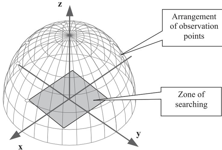
Fig. 2. Arrangement of sound sources and observation points on the surface of the semi-sphere.
