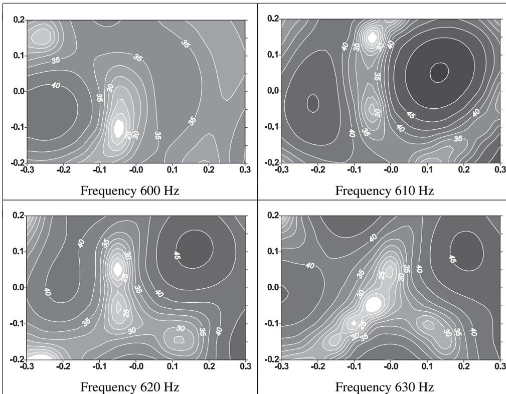
Fig. 10. Power level of the substitute sound source in a bandwidth of 2 Hz.
