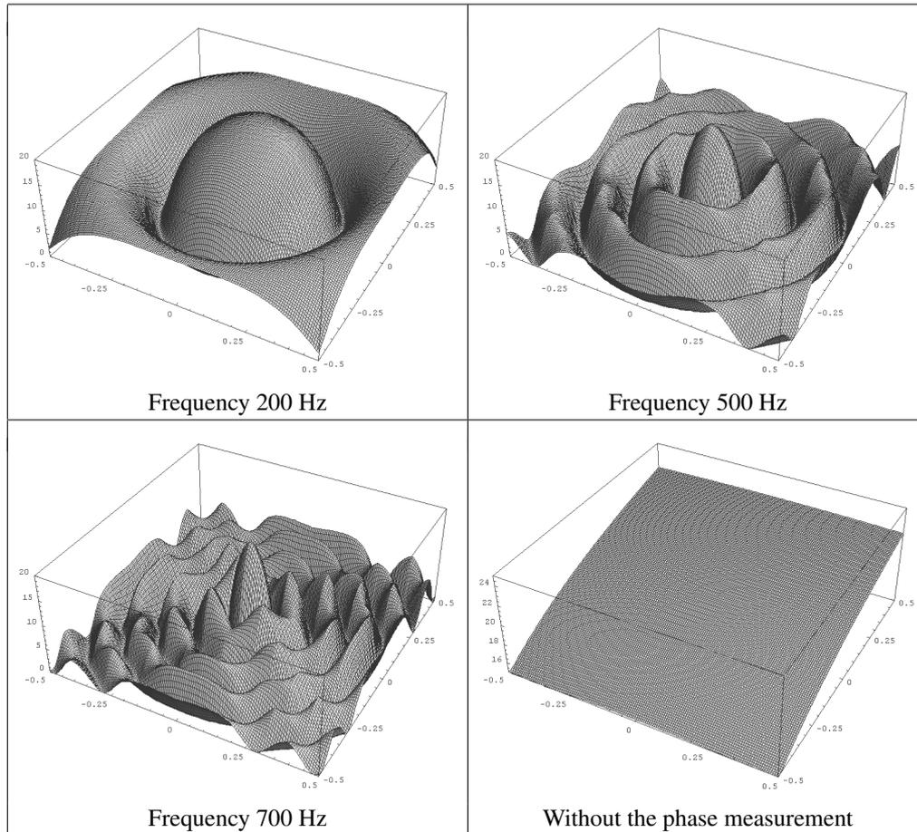
Fig. 7. Sound power levels of the substitute source depending on its position – observation points arranged on the straight line.
