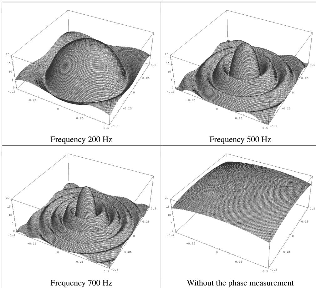
Fig. 3. Sound power level of the substitute source depending on its position – observation points arranged on the surface of the semi-sphere.
