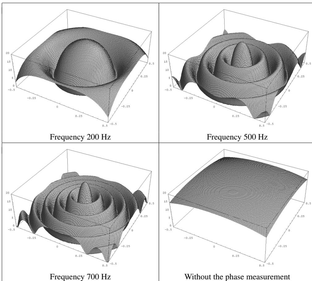
Fig. 5. Sound power level of the substitute source depending on its position – observation points arranged on the circle.
