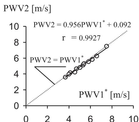
Fig. 8. Pulse wave velocity (PWV) in the CCA for the group of people examined:  $PWV1^*$  – determined on the basis of measurement of variation of the diameter CCA and blood pressure in the BA (Eq. (3)) under the assumption that the diastolic and mean blood pressure in the CCA are the same as in the BA;  $PWV2$  – determined on the basis of the blood flow velocity measured at two points.
