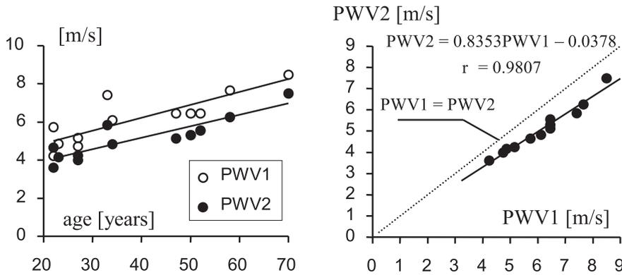
Fig. 4. Pulse wave velocity (PWV) in the CCA for the examined group: PWV1 – calculated from formula (3), PWV2 – measured on the short artery segment.
