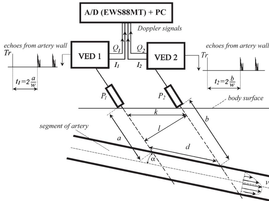
Fig. 1. Experimental setup:  $k, l$  – distances between the axes of ultrasonic beams of probes P1 and P2,  $w$  – velocity of ultrasonic waves,  $t_1/2, t_2/2$  – times of the ultrasonic pulse propagation between the probes P1, P2 and the anterior surface of the carotid wall,  $\alpha$  – angle between the ultrasonic beams and the axis of the artery ( $0^\circ < \alpha < 90^\circ$ ).
