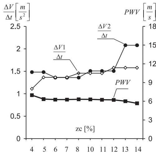
Fig. 3. The increase of the blood velocity in time  $\Delta V/\Delta t$  for the initial part of systolic phase for measurement points 1 and 2 and local PWV for different increases of blood flow amplitude levels  $zc$ . Results concern a man 58 years old.  $PWV = 6.6 \text{ m/s}$  for  $\Delta V1/\Delta t \approx \Delta V2/\Delta t$ .
