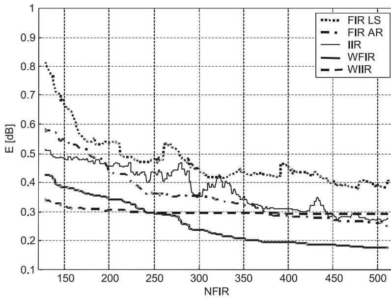
Fig. 6 Standard deviation of magnitude response versus equalizing filter order. Analysed band: 100 Hz-8 kHz. Loudspeaker system no. 2.
