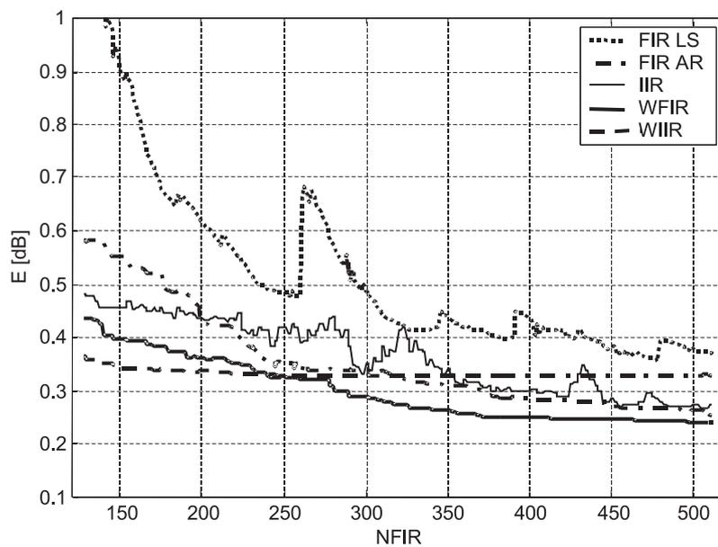
Fig. 5 Standard deviation of magnitude response versus equalizing filter order. Analysed band: 63 Hz–20 kHz. Loudspeaker system no. 2.
