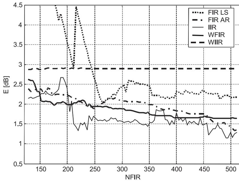
Fig. 2 Maximum magnitude response irregularities versus equalizing filter order. Analysed band: 77 Hz–20 kHz. Loudspeaker system no. 1.
