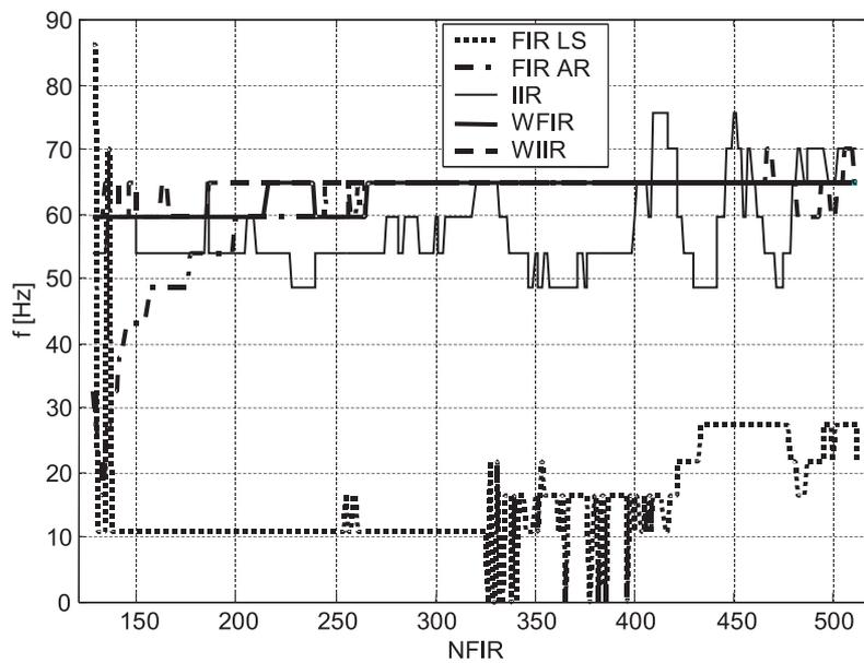
Fig. 7 Lower response frequency during preprocessing, allowing one to obtain an assumed lower frequency-range frequency after equalization. Loudspeaker system no. 2.
