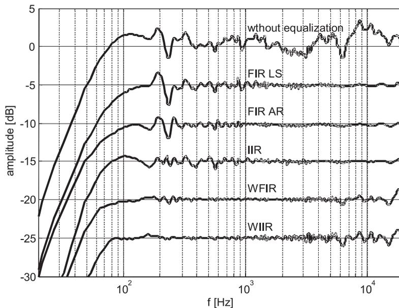
Fig. 8. Comparison of magnitude responses before and after equalization for the loudspeaker system no. 2.
