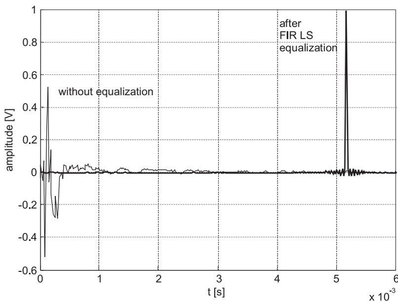
Fig. 9 Impulse response of loudspeaker system no. 1 before and after equalization by means of filter FIR LS.
