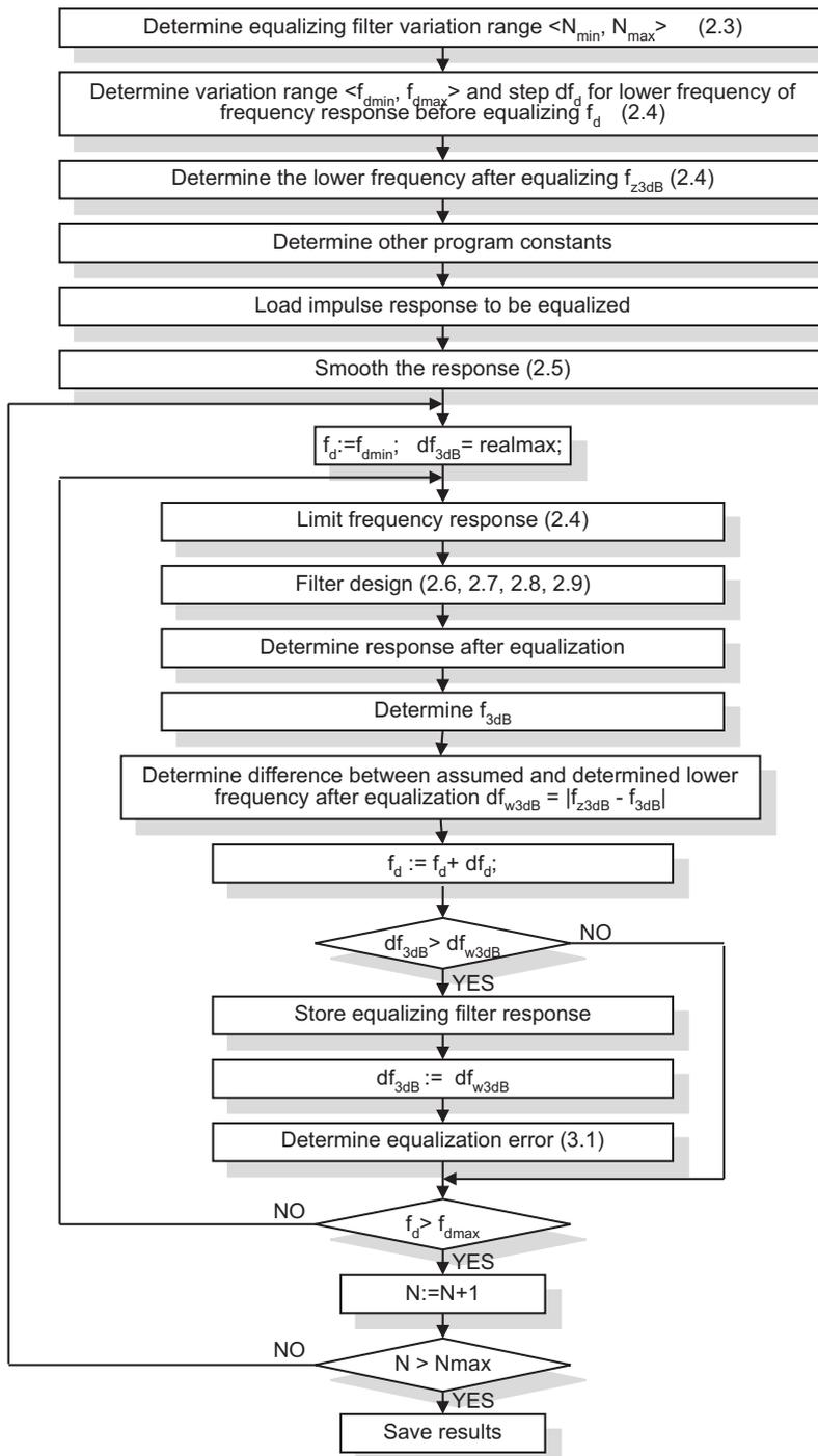
Fig. 1. Equalizing filter design algorithm.
