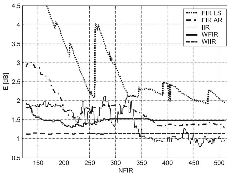
Fig. 3 Maximum magnitude response irregularities versus equalization filter order. Analysed band: 63 Hz–20 kHz. Loudspeaker system no. 2.
