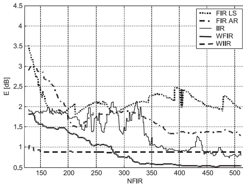
Fig. 4 Maximum magnitude response irregularities versus equalization filter order. Analysed band: 100 Hz–8 kHz. Loudspeaker system no. 2.
